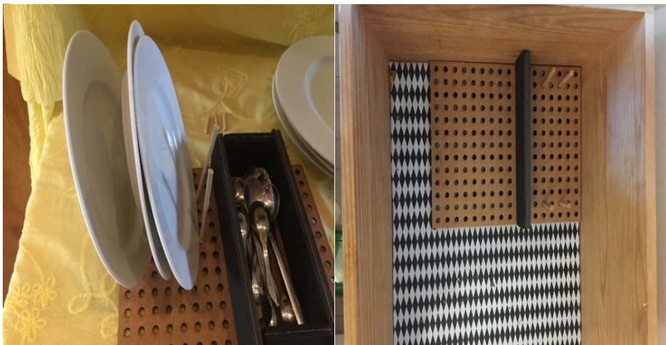
Figure 3.3 Testing of the first experimental prototype in the drawers and bearing the plates.
