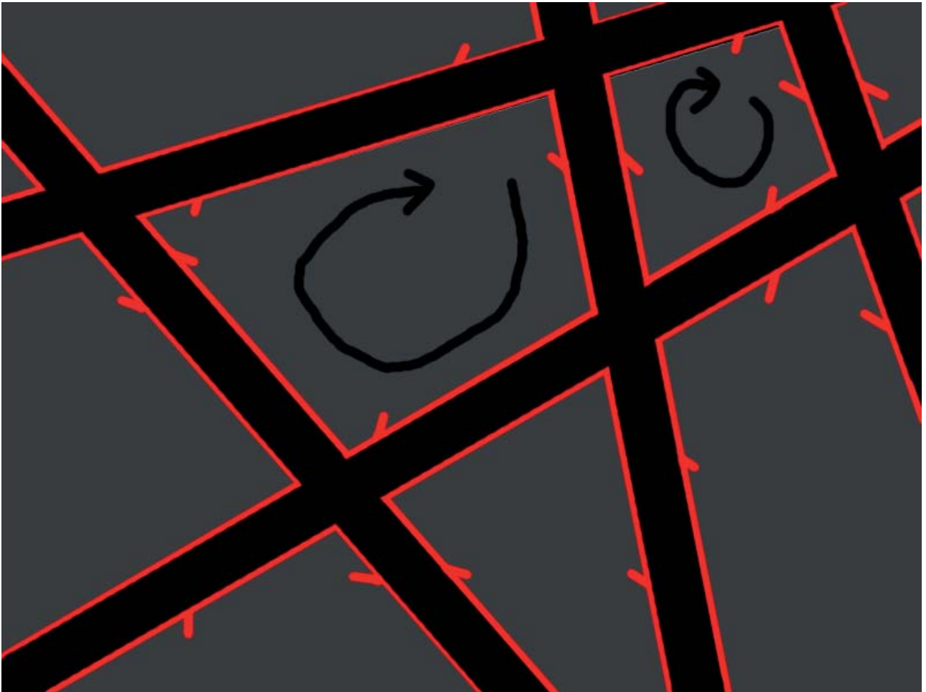
Figure 8: Lines are checked for collisions against each other, intersection points are saved as polygon points. Each line keeps track of potential parent line and child line.
