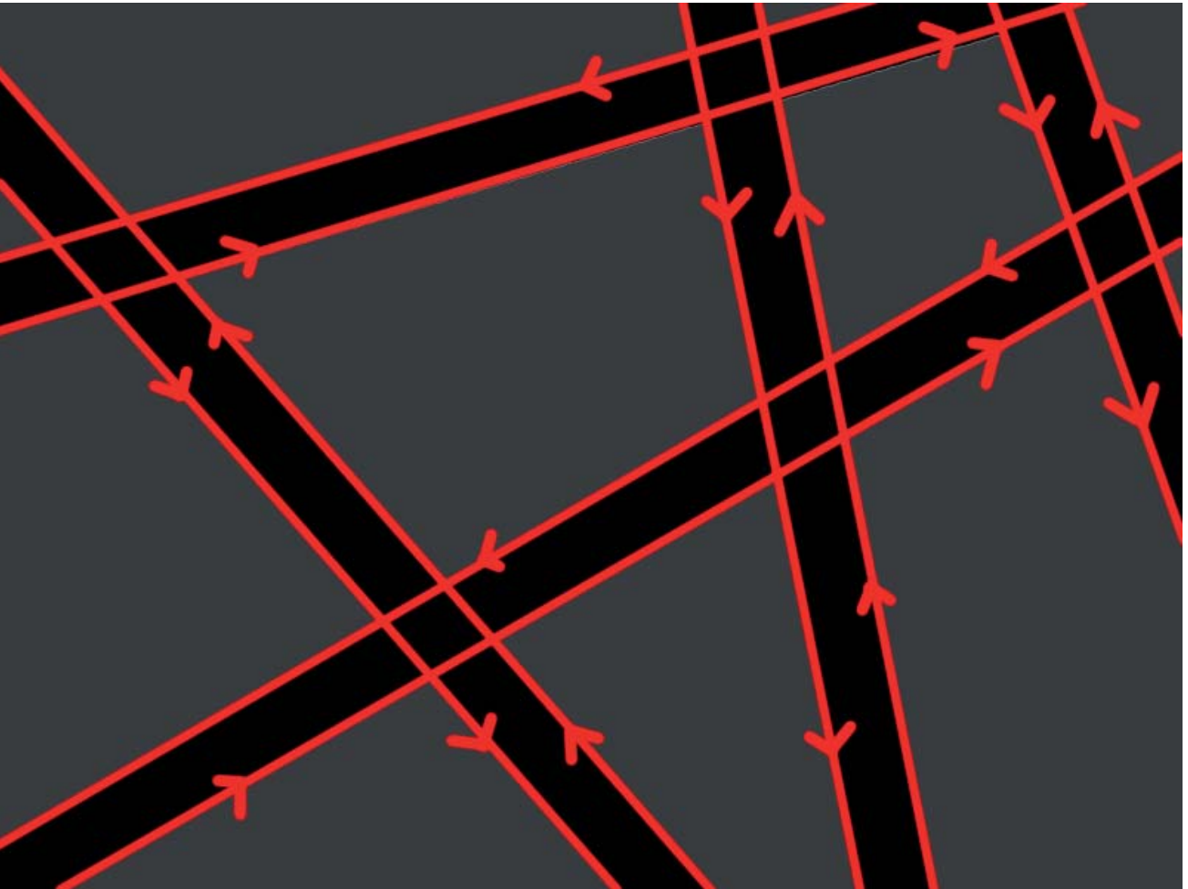
Figure 6: Roads with lines placed on both sides, direction is reversed for opposing sides
