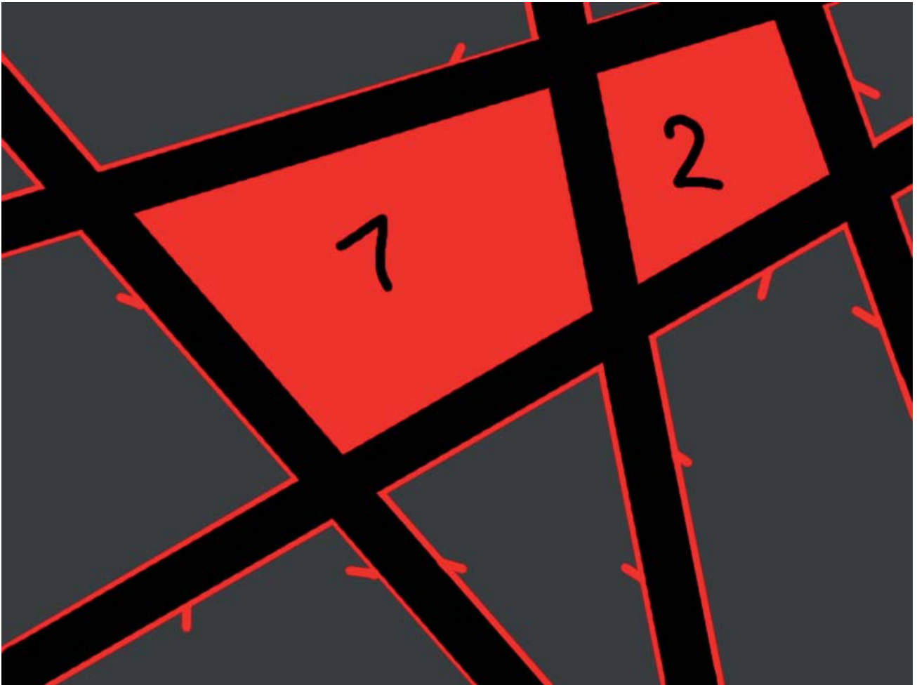
Figure 9: In every polygon where the last point has the first point as child, a complete polygon and is formed and saved. In this limited example, two polygons are created
