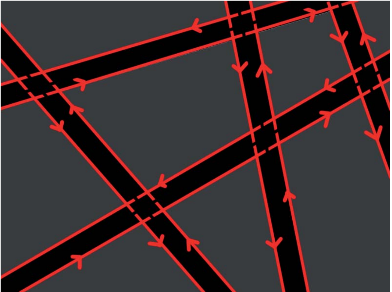
Figure 7: Lines are split whenever intersecting the middle of a road, recursively creating new lines
