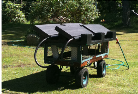
Image 1. Compotherm, mobile solar water-cleaners.
