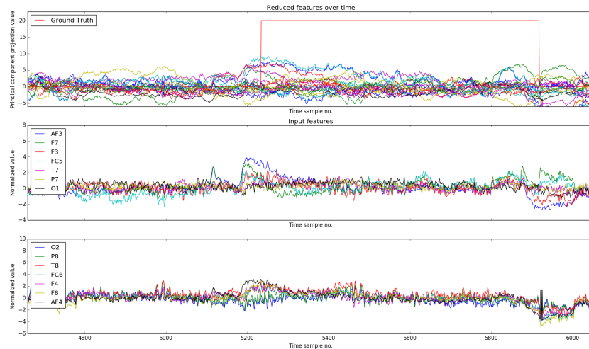
Figure 40: A section of the Eye data set, aligned with the corresponding reduced features generated by the Component ESN. We can see that a short-time spike in the input features results in a long "echo" in the generated features. This seems to be a good rule, if one looks at the input data.
