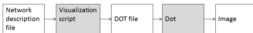
Figure 3.2: The workflow for generation of topology images. The shaded boxes represent programs, and the white boxes represent files.
