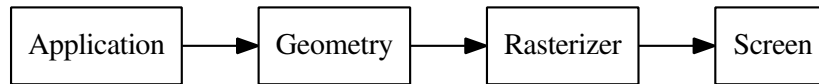
Figure 1.1: This figure shows the three major steps of the graphics rendering pipeline. For clarity, a screen has been added to the figure, even though it is not part of the pipeline.
