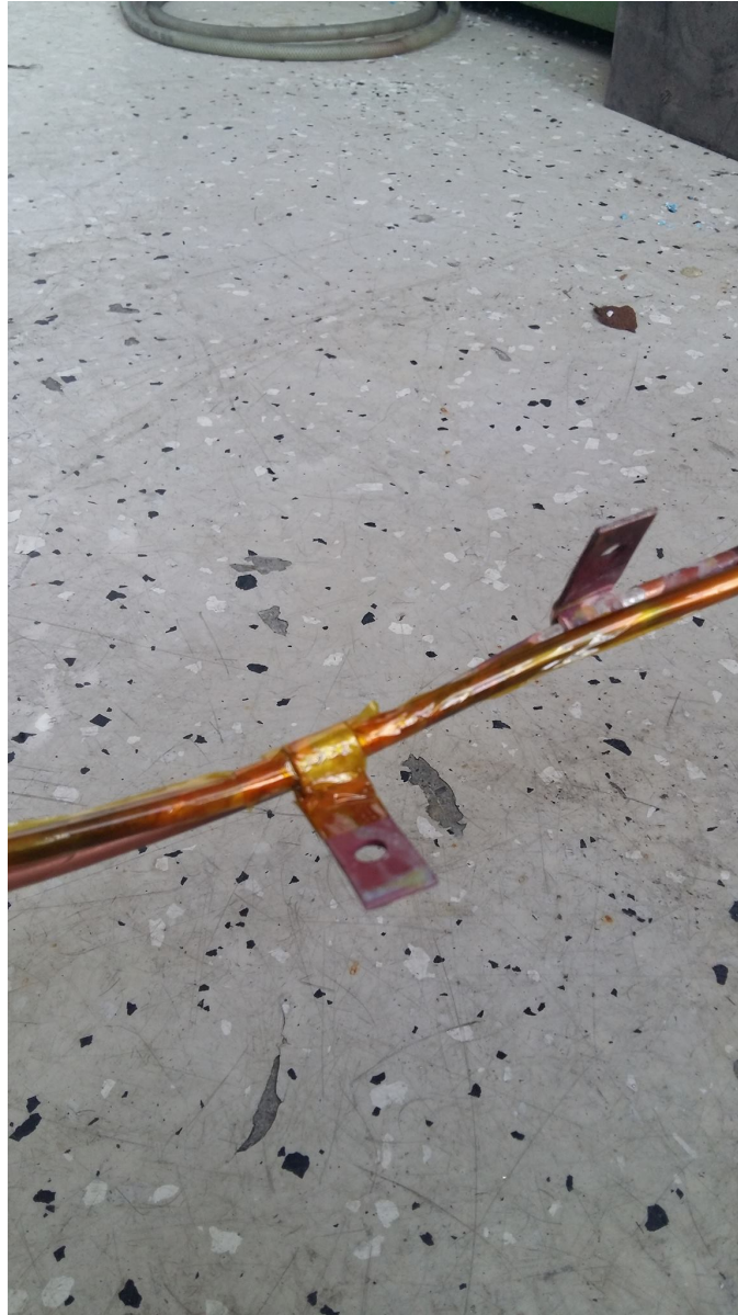
Figure 84: Power supply fittings brazed on to the copper tubing
