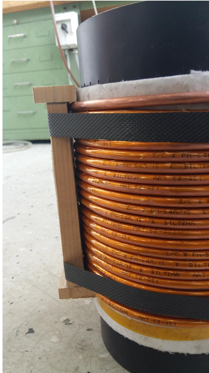
Figure 86: One of the mounted wooden racks
