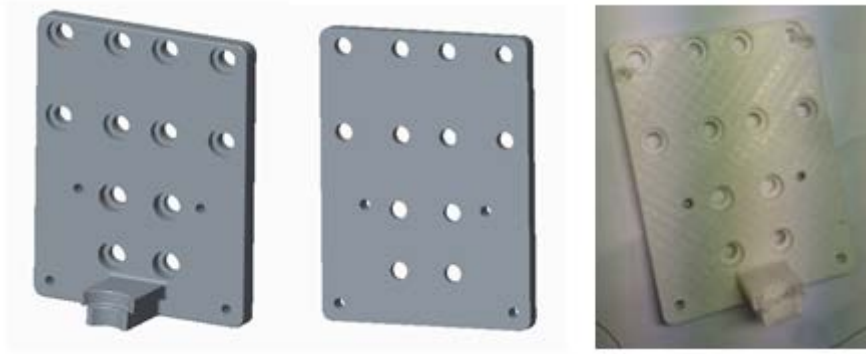
Figure 8, design of mounting bracket
