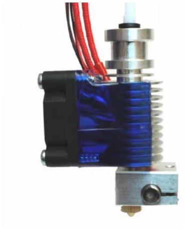
Figure 12, design of hot end
