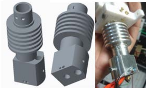
Figure 19, Design of new extruder
