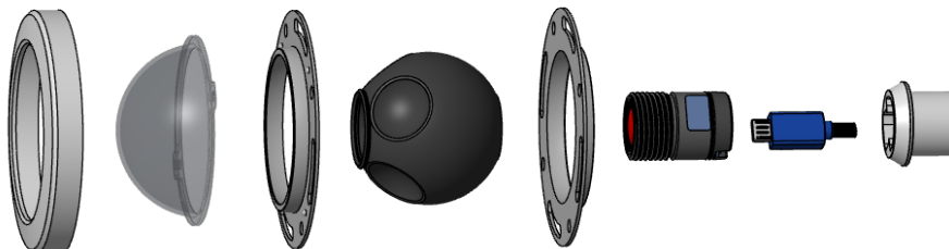
Figure 14.5 CAD model of the exploded view of the Mini Silicone concept.
