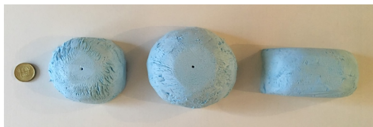
Figure 13.1 Prototypes in Styrofoam. From right to left: Ø70 mm, Ø90 mm, 90 x 45.
