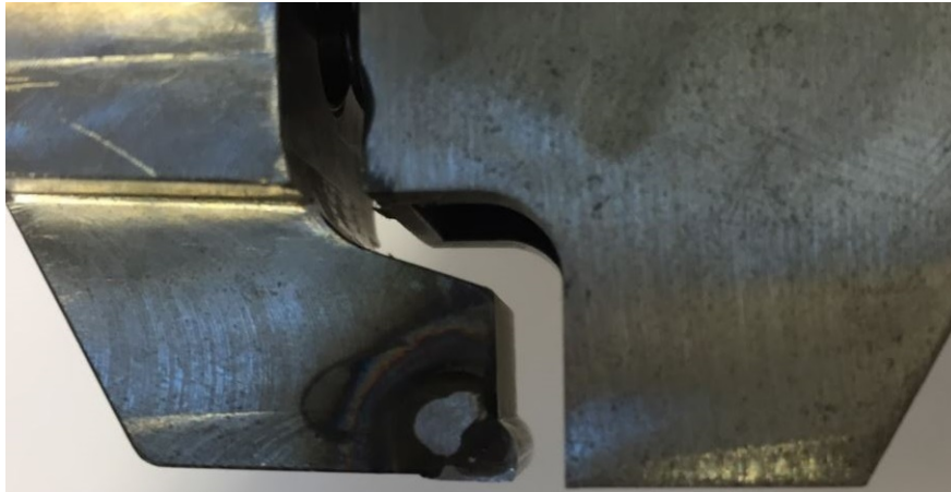
Figure 3.1: The upper clamp used in the tensile tester at Tetra Pak.
