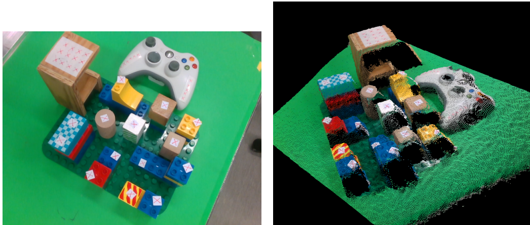
(a) A scene visualized using a regular 2D image. (b) The same scene visualized as a point cloud.
