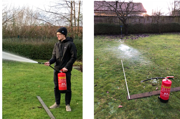
Figure 3.4: Testing a fire extinguisher with foam as extinguishing agent to measure its reach and capacity
