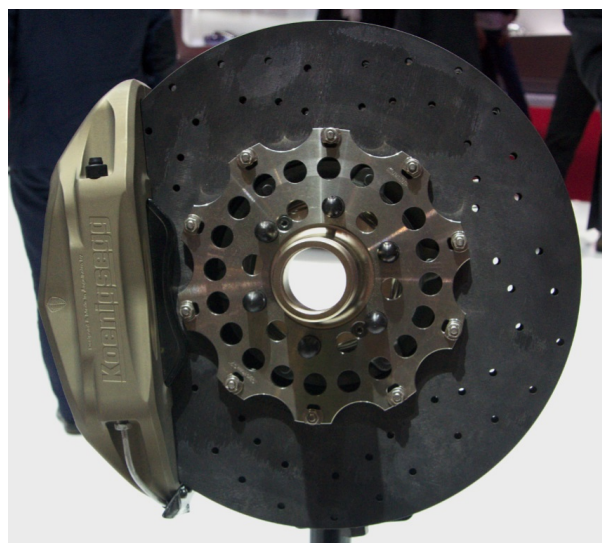
FIGURE 1.2: Disc brake of a high-performance car [F2]
