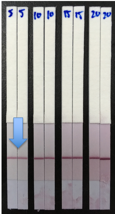
Figure 10. Showing the resulting test line intensity after addition of different volumes of detection antibody with the concentration 0.12\mu\text{g}/\mu\text{l} . From the left in duplicates: 5, 10, 15 and 20 \mu\text{l} . The optimal volume was determined to be 5\mu\text{l} (see blue arrow). Antigen concentration in test line was 2\mu\text{g}/\mu\text{l} .
