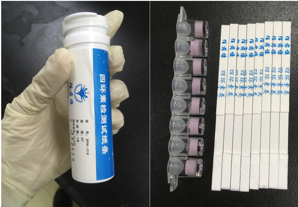
Figure 20. Showing the finished product and its distribution. Each plastic desiccant bottle (left) containing a set of eight covered microwells with freeze-dried components and eight test strips (right).
