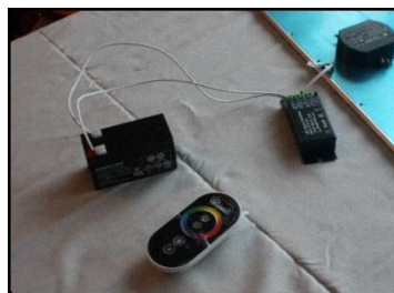
Figure 3-11 Battery (left) attached to a receiver, in turn attached to the LED-strip.
