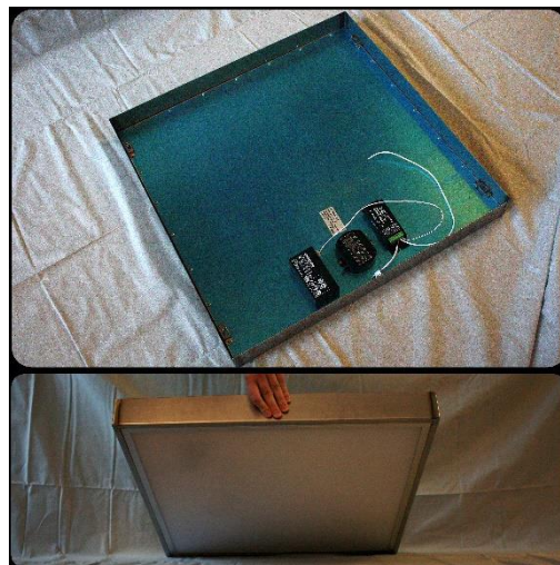
Figure 3-15 Ceiling prototype fitted inside steel frame
