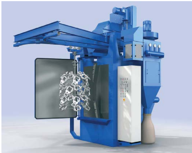
Figure 73: Hanger blasting machine. [22]
