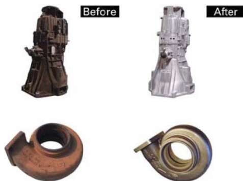
Figure 74: Before (left) and after (right) slurry blasting. Upper: Gearbox housing. Lower: Turbo housing. [24]
