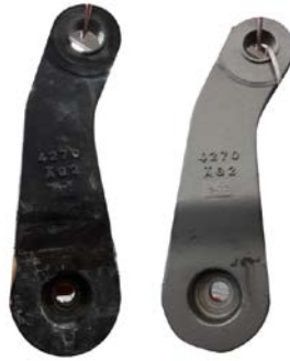
Figure 72: Comparison of before and after blasting in the hanger blasting machine. Left: Before. Right: After
