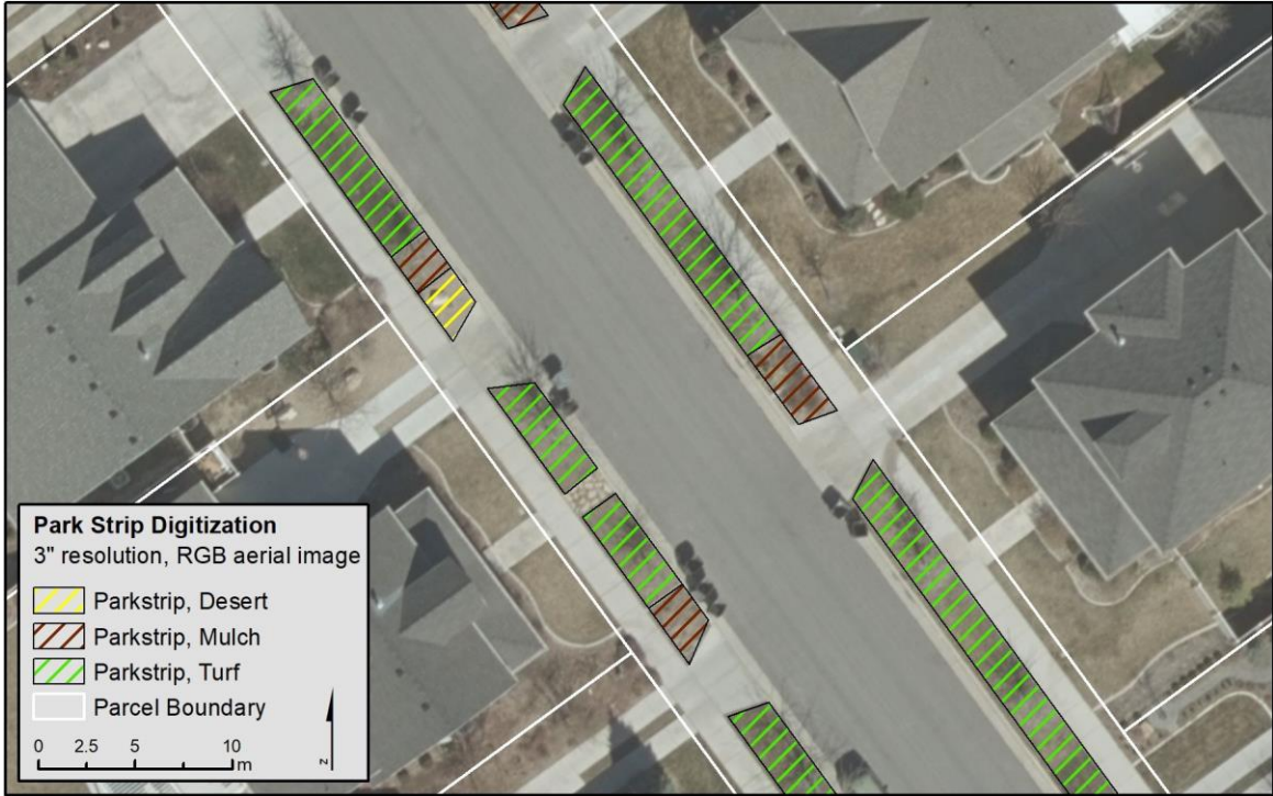
Figure 11: Park strip land cover digitization and classification - 2017 aerial image, 3 inch per pixel resolution
