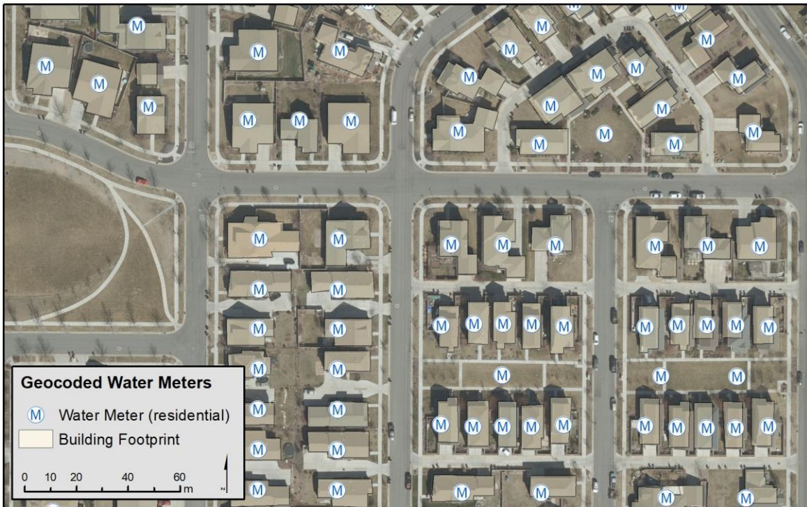
Figure 4: Geocoded residential water meters
