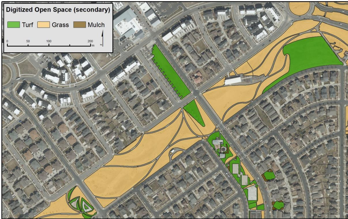
Figure 8: Manually digitized areas irrigated with secondary water based on the provided DWC map
