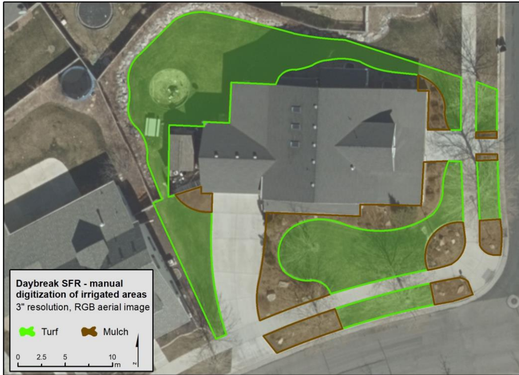
Figure 14: manual digitization and ground cover classification of irrigated areas for a selected sample lot based on 3in resolution aerial image
