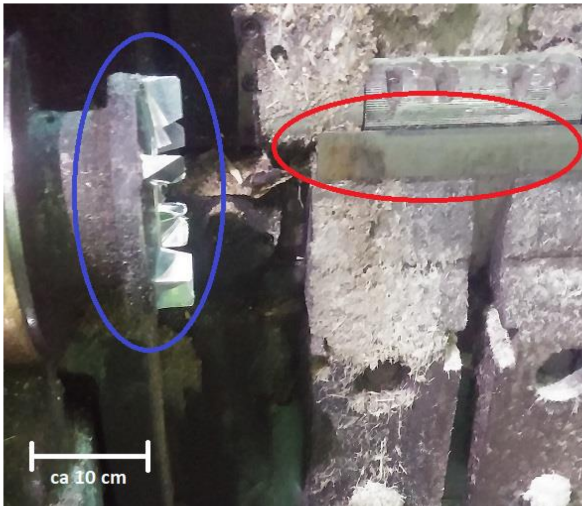
Figure 3.2.2 Left chuck, marked with blue, and part of the knife, marked with red, after cleaning for sharpening.
