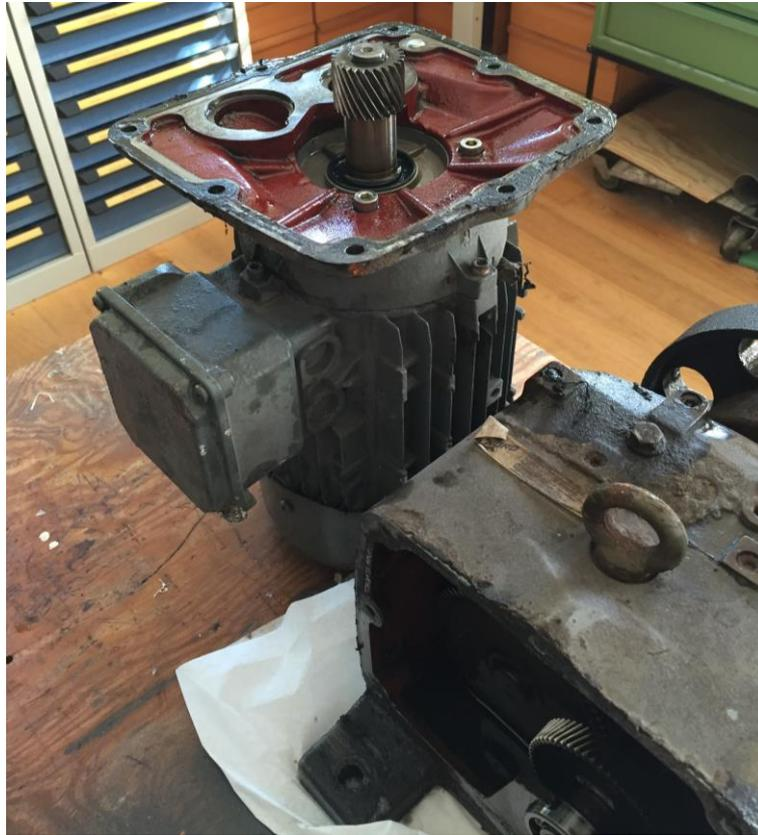
**Figure 4.16 Motor separated from gearbox.**
