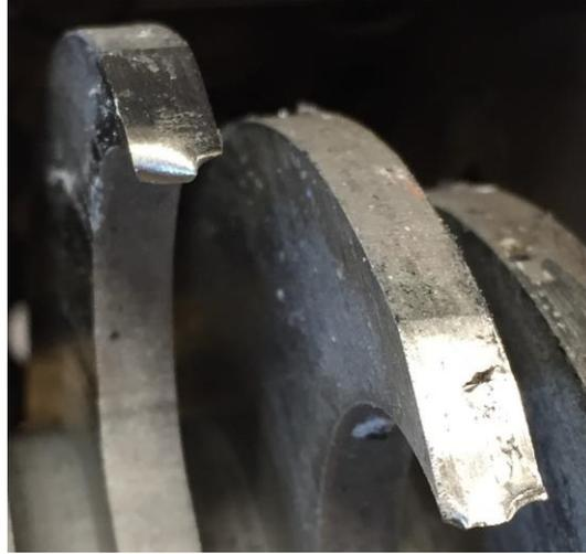
**Figure 5.6 Chipping of the teeth after testing the shredder.**
