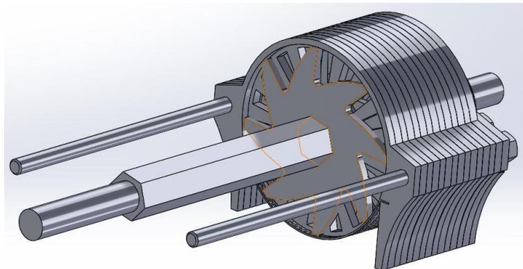
Figure 6.14 Final redesign - exploded view.
