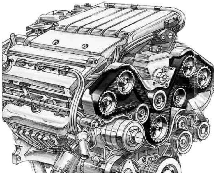
**Figure 4.11 Ribbed belt as a timing belt for the camshafts of a car engine.**
