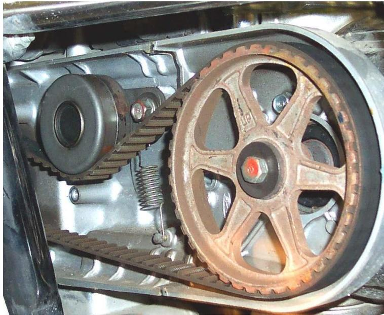
**Figure 4.12 Spring tensioner on a ribbed belt.**
