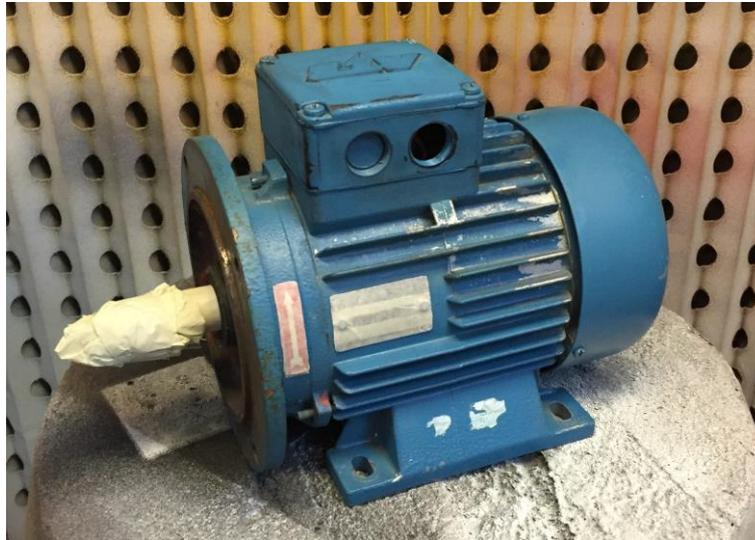
**Figure 4.27 Motor prepared for primer and paint.**
