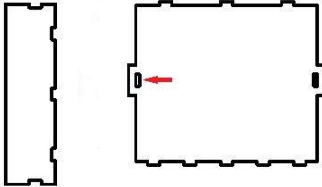
**Figure 3.3 Two pieces with puzzle shaped connectors. Slits dependent on sheet metal thickness marked by arrow.**
