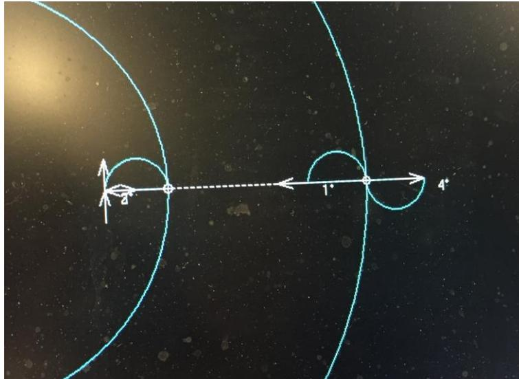
**Figure 4.30** Double lines that cause double engaging points as seen on the rightmost line. The object to be cut is a ring between the two lines. The blue lines represent the cutting path of the waterjet cutter.
