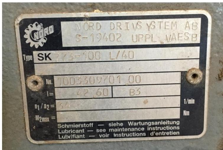
Figure 4.14 Rating plate on the gearbox.
