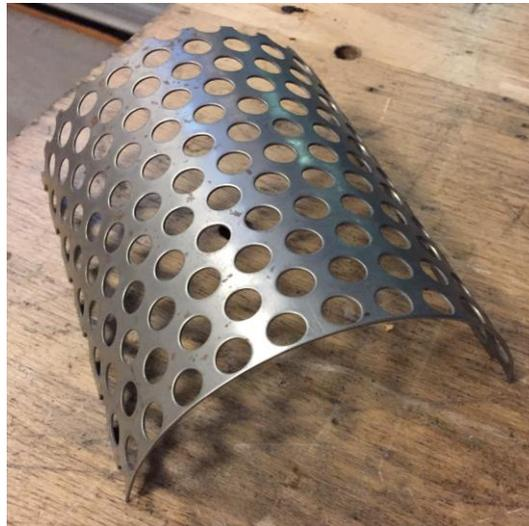
**Figure 5.4 Sieve with a larger perforation.**
