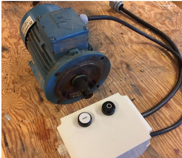
**Figure 4.7** Motor connected to a protective circuit breaker.
