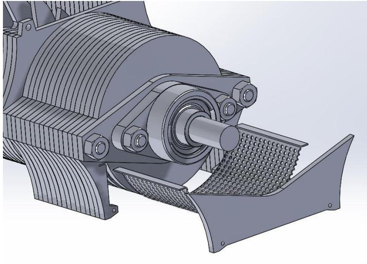
**Figure 6.11 Exploded view of the redesigned mesh assembly.**
