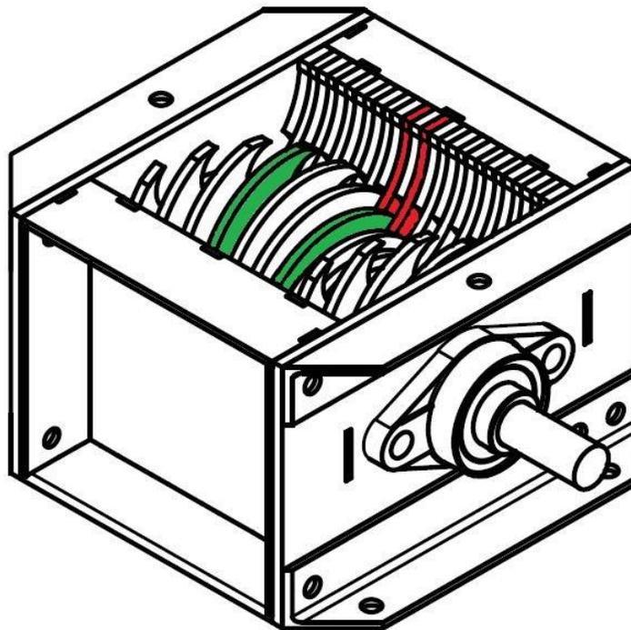
Figure 3.2 SSP where knives (green) and counterknives (red) are marked.
