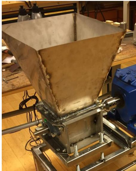
**Figure 4.37 The hopper when mounted on the SSP.**
