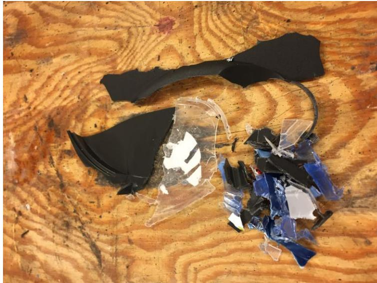
**Figure 5.2 Different sizes when shredding without a sieve.**
