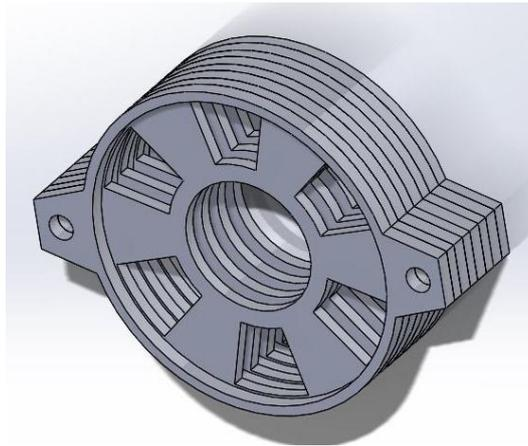
**Figure 6.6 Integrated housing with spacers and counterknives.**
