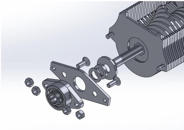
Figure 6.9 Exploded view of redesigned bearing assembly
