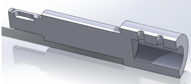
**Figure 4.24 CAD model of the lathed shaft with an intergrated connector.**
