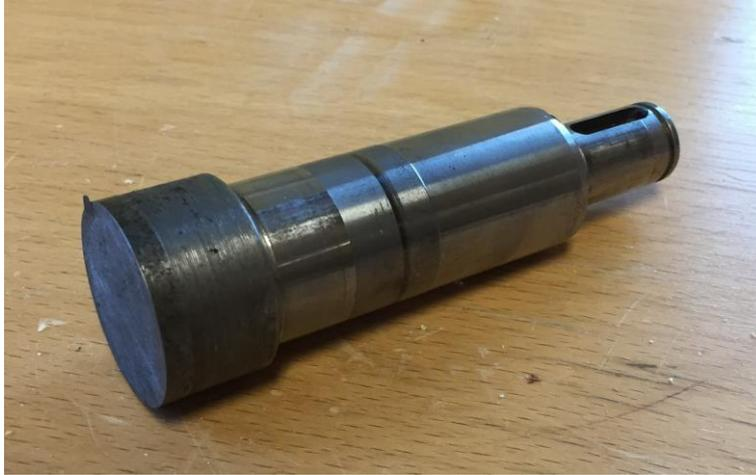
**Figure 4.22** The gearbox motors shaft after cutting off the rotor and removing the flange and helical gear.
