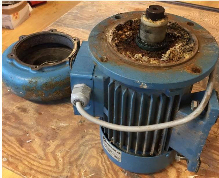
**Figure 4.6** Motor after removing the pumphouse and part of the impeller.
