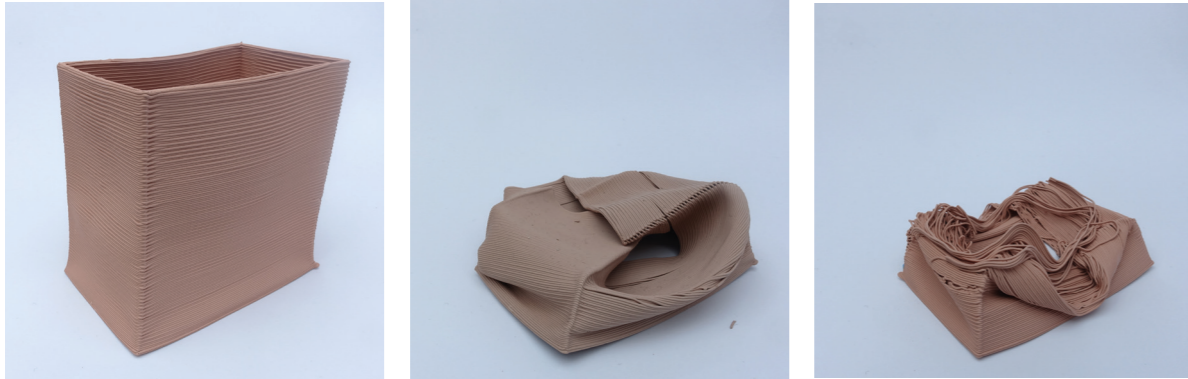
The four cornered model is printed at 100% speed, 200% speed and 300% speed. The collapse happens in the corners.
