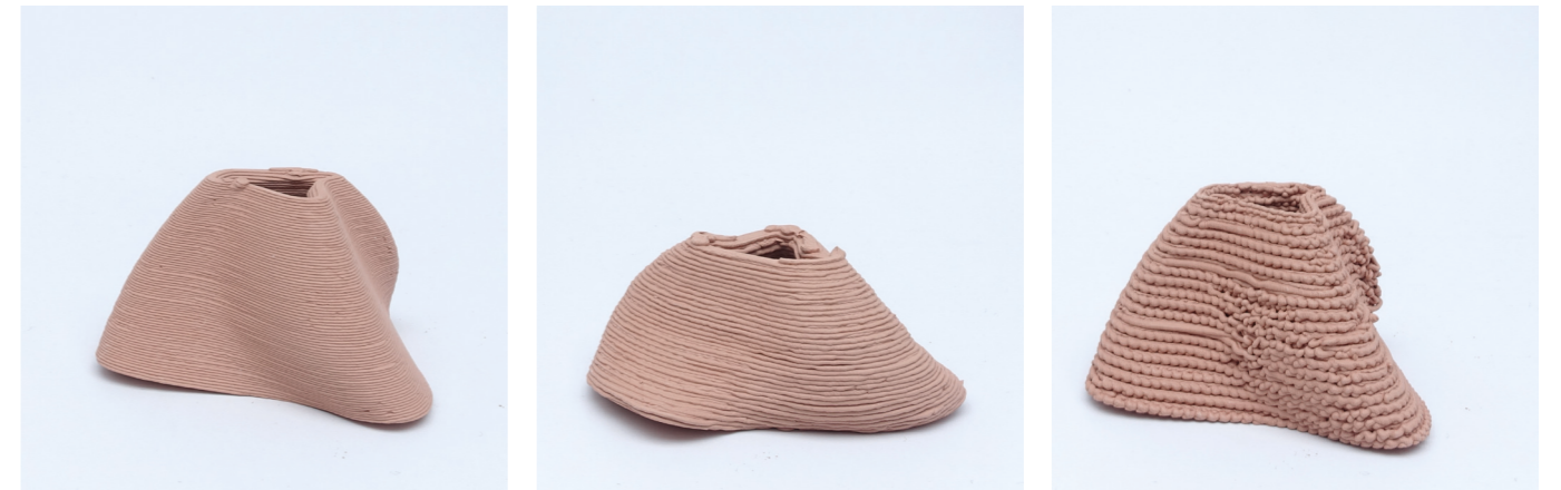
Changing the layer height affects different models differently. Here are layer height 0.4 mm, 0.8 mm, 1 mm.
