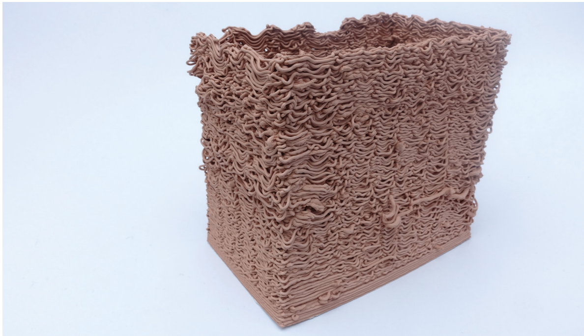
In the four cornered model 0.8 mm layer height and a slower printing speed is creating a pattern similar to 1 mm layer height in the model with a curved wall.
