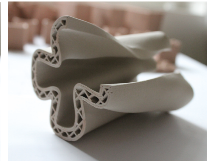
The curved continuous surface, the infill and the two millimeter shell thickness is what creates stability in this model.
