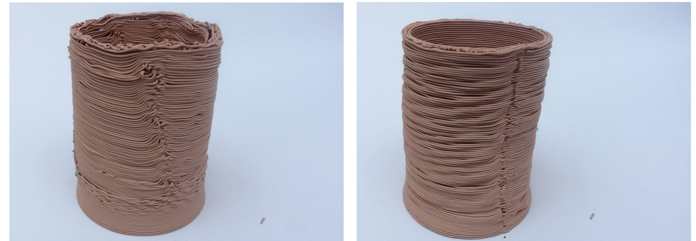
Print speed also affect the print. The right model is printed at double speed from the left model.
