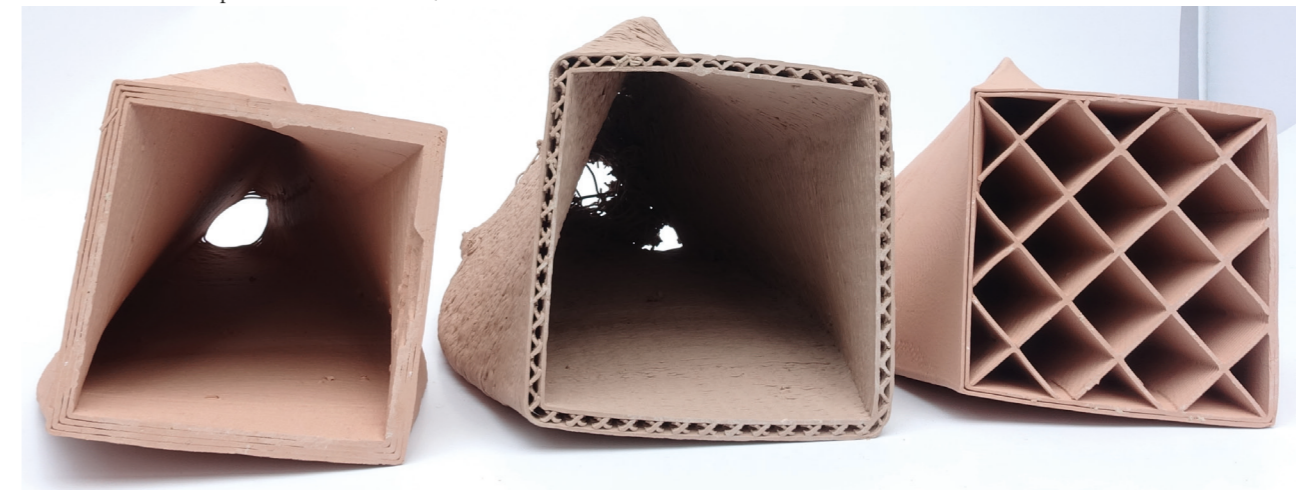
The first model has 4 mm shell thickness, the second has 1 mm shell combined with infill, the third has 2 mm shell and infill.
