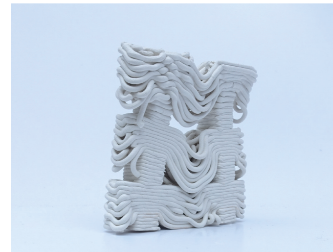
The straight walls from the computer models are crumbling when faced with reality.
