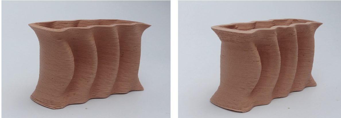
The right model is printed at 250% of the speed of the left model and little difference can be seen between the two.
