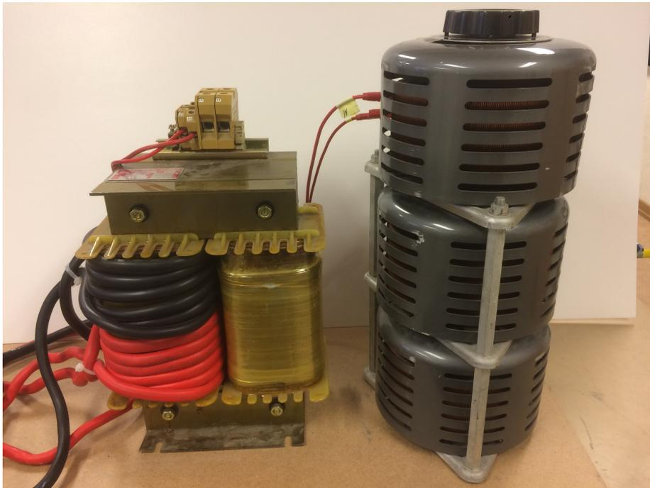
Figure 24: The transformers used to generate the required heat loads.
