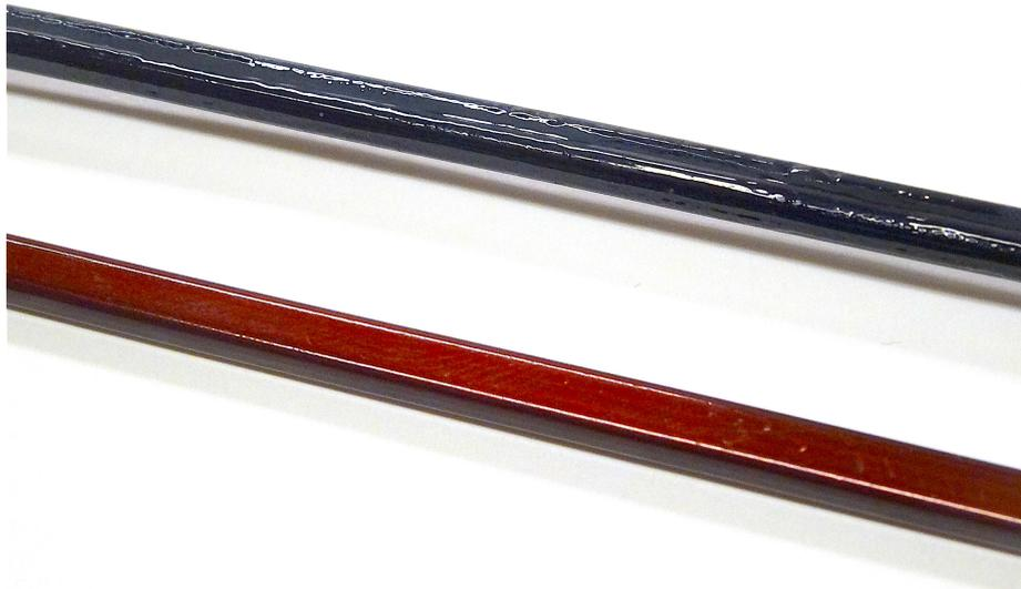
Figure 43: Copper insulation subjected to  $\sim 250^{\circ}\text{C}$  next to unused conductor.
