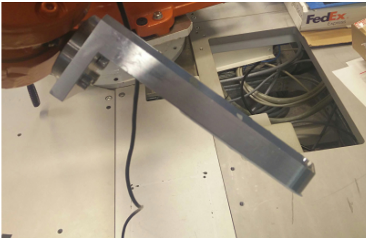
A.10 The pen holder seen from its left side with the cover and screws removed.
