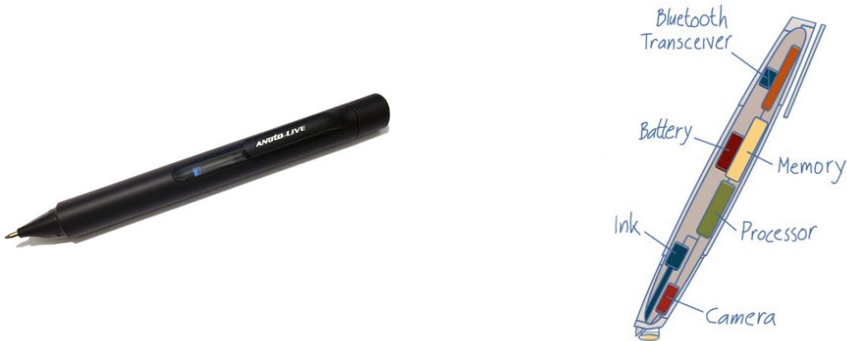
Figure 2.3 To the left: The Anoto Live pen with active display [Xms Penvision, 2017]. To the right: A generalized drawing of the components in the pen [NECS, inc, 2017]. The infrared emitting diode and force sensor are not annotated in the figure.
