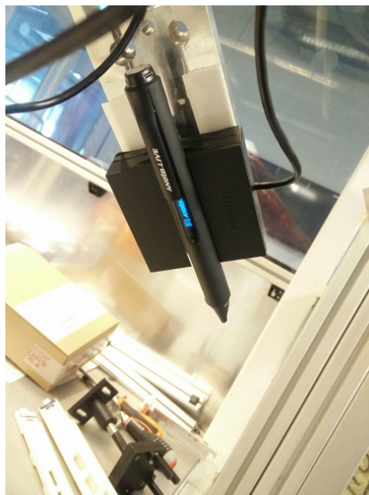
A.16 An Anoto Live pen with its cradle attached on the adhesive tape on the pen holder.
