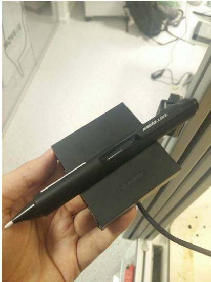
A.8 An Anoto Live pen in its cradle with its digital display turned off.
