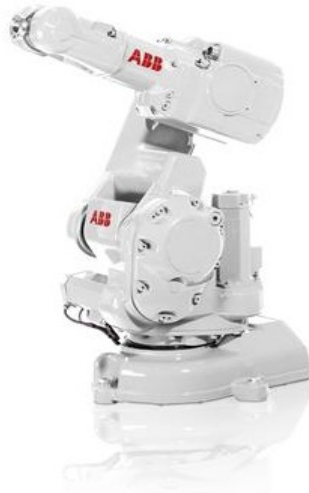
Figure 2.4 The 6 DOF IRB140 robot manipulator from ABB [ABB Ltd, 2016c].
