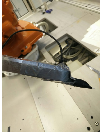
A.20 A prototype pen fastened firmly with duct tape seen from its left side.
