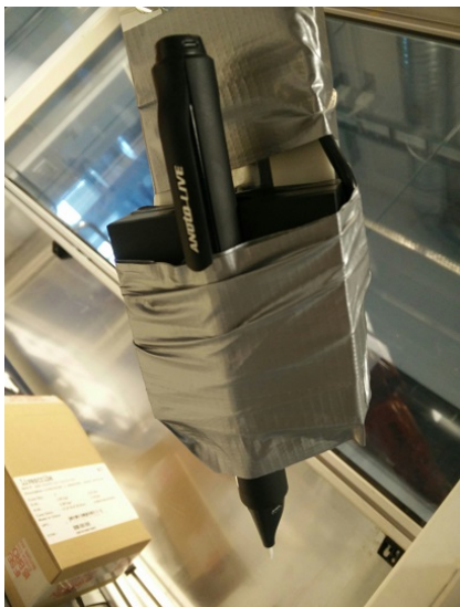
A.17 An Anoto Live pen and cradle fastened firmly with duct tape seen from its top side.
