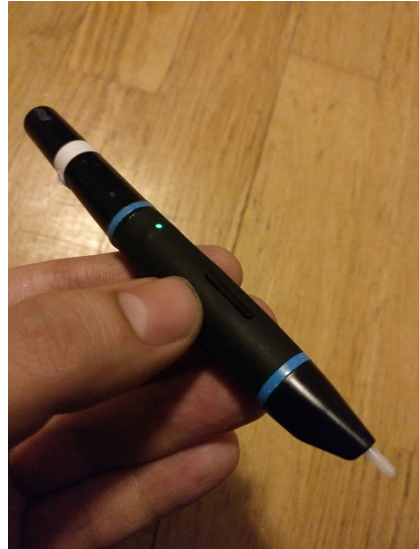
A.9 A prototype pen with its green status LED active.
