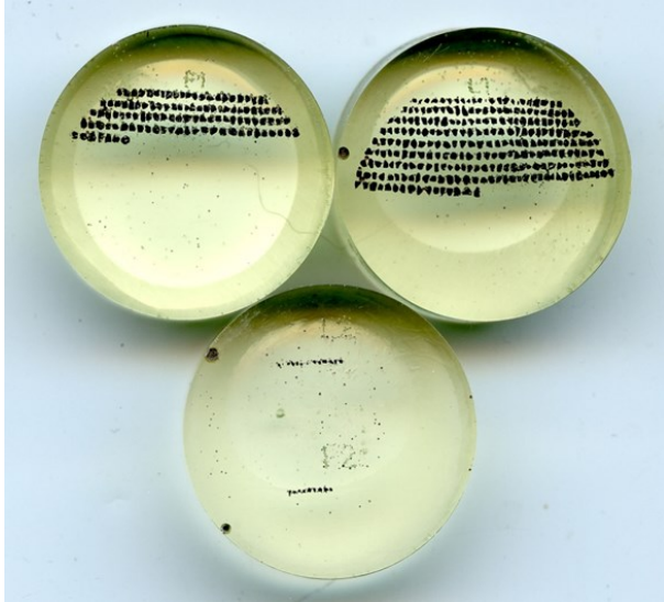
Fig. 15. Pyrite samples, F1 (top left), L1 (top right) and L2/F2 (bottom), in hardened epoxy.
