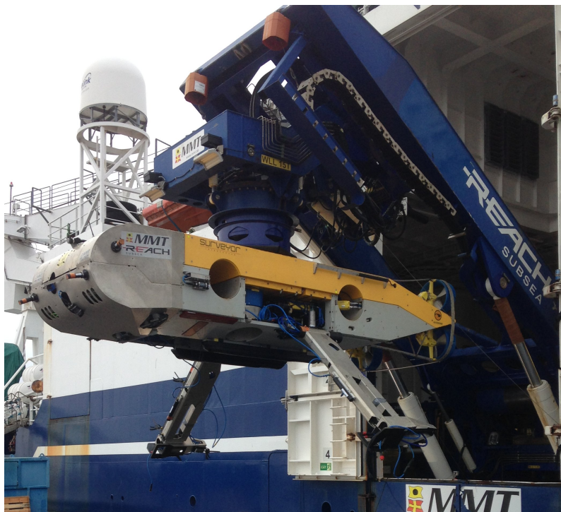
Figure 1.1 Photography of the SROV used for the trials on Stril Explorer.
