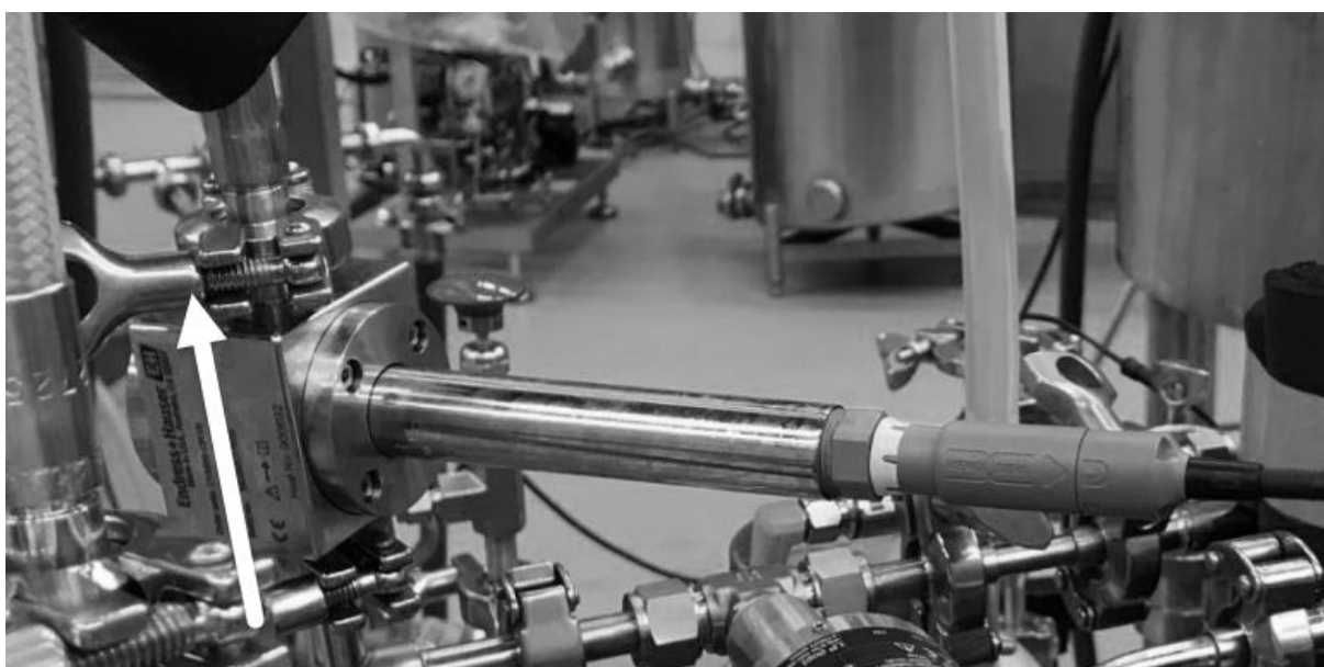
Figure 3.5. The positioning of oxygen sensor denoted “OT02” in the flow diagram with the flow direction marked with the arrow.
