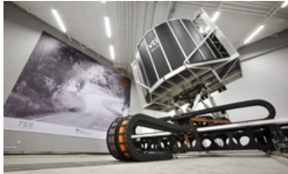
Figure 1.4: The tiltable car cabin
