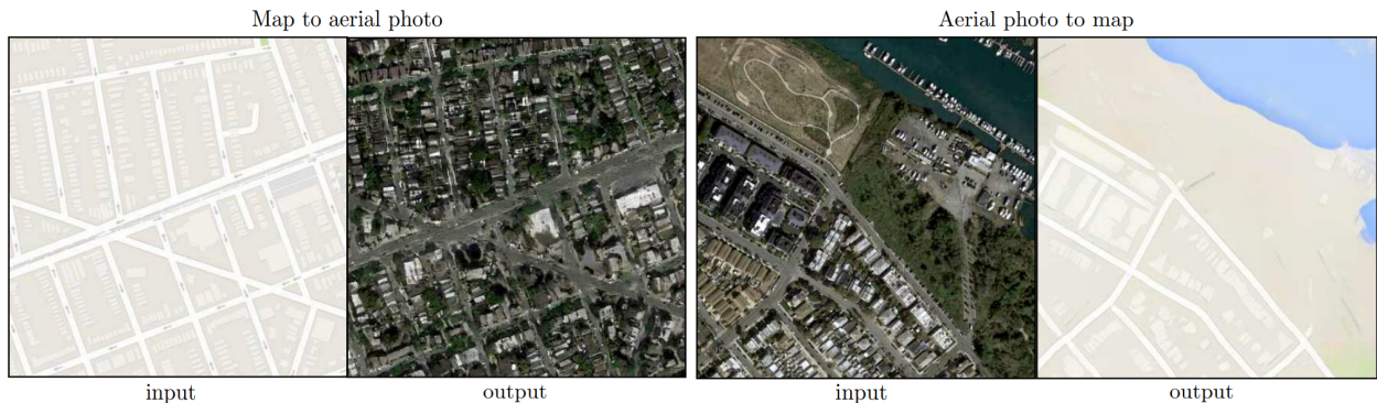
Figure 19: Results from training Pix2Pix on paired images of maps and aerial photos. In the left part of the figure the network is trained to generate an aerial photo given a map as input. In the right part the problem is reversed, the network is trained to generate a map given an aerial photo as input.
