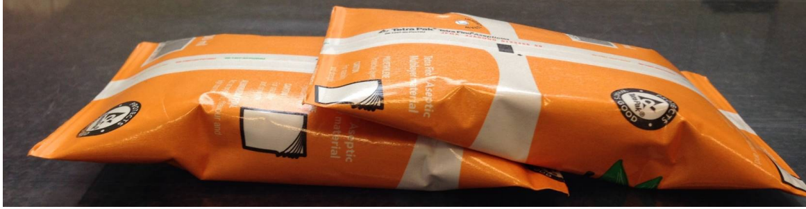
Figure 3.3: Test setup for overlap testing. P1 is put in the bottom (left in image) and P2 on top (right in image). 50% overlap is shown in the image.
