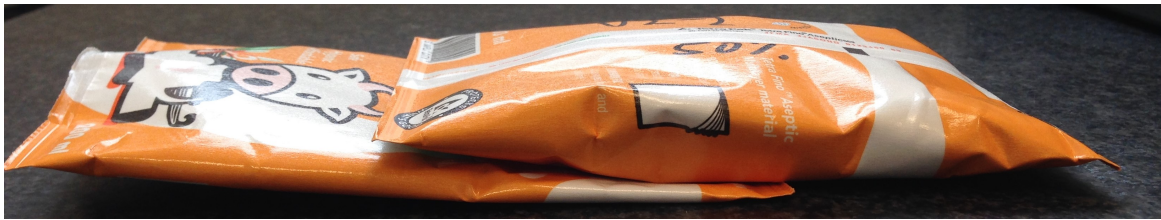
Figure 5.6: Typical state after rupture for overlap test.
