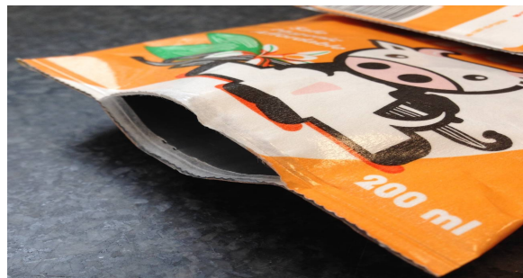
Figure 5.7: Rupture of P1 after compression test using overlap.
