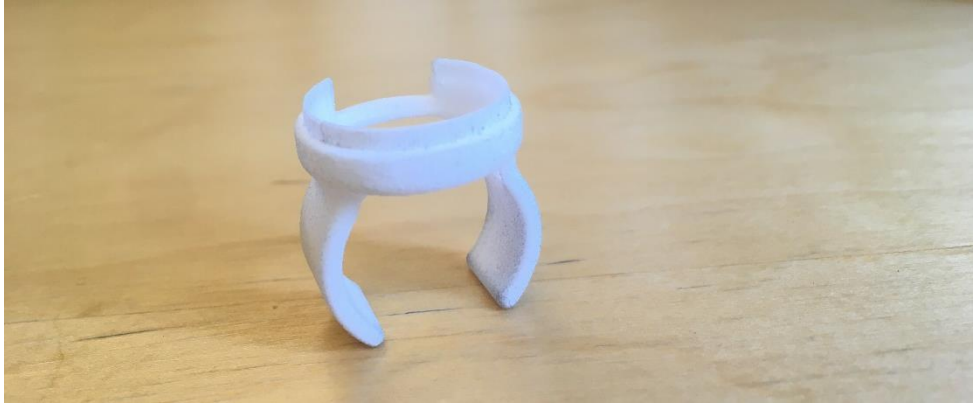
Figure 73 Picture of the SLS printed prototype
