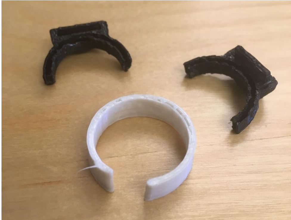
Figure 53 The three 3D-printed parts that make the flexi ring prototype
