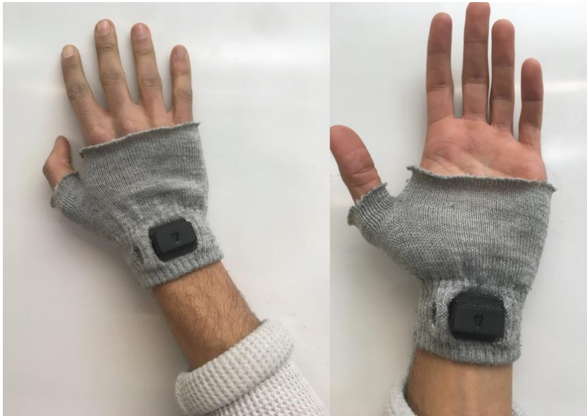
Figure 32 Lo-fi prototype created by combining 3D-printing and fabric
