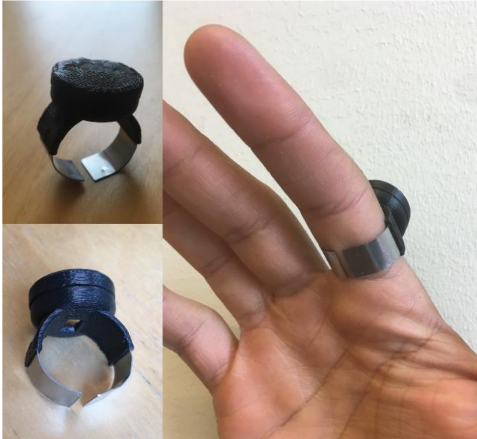
Figure 61 Prototype of flexi ring made with spring steel
