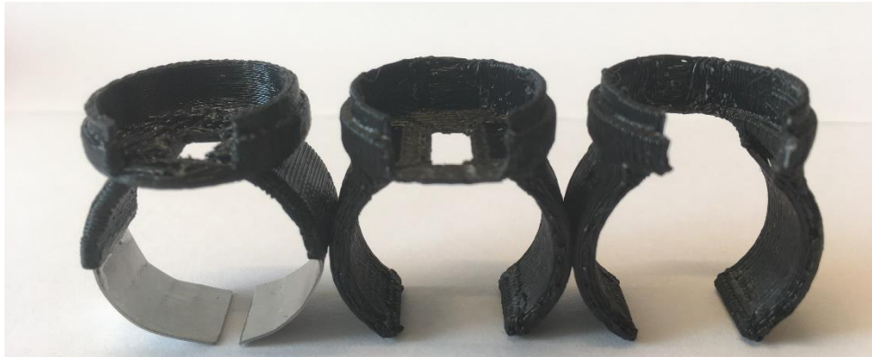
Figure 66 Illustration of the different “floor” thicknesses. To the left, 1.5 mm thick. In the middle 0.6 mm thick. To the right 0 mm thick
