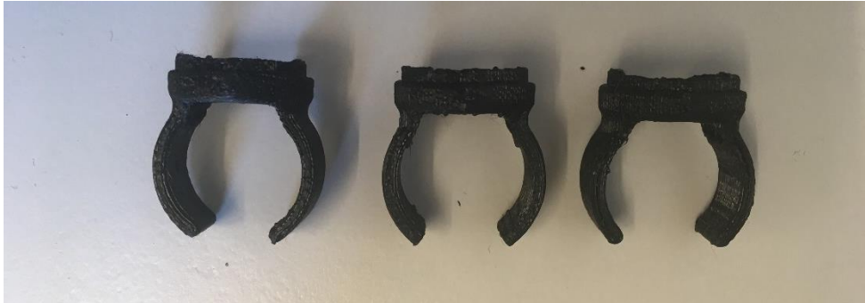
Figure 65 Prototypes created to investigate the angle of the open ring. From the left; 60°, 70° and 80°
