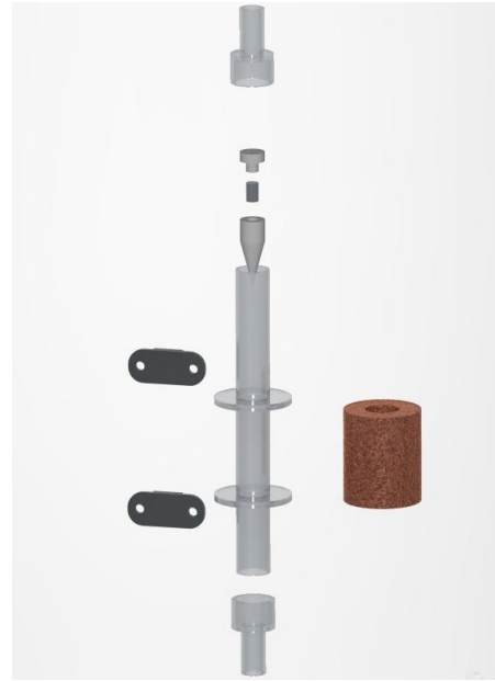
FIGURE 3.19: Final design of the sensor, exploded view.
