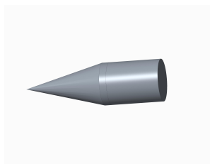
FIGURE 3.3: Cone float with cylindrical extension.
