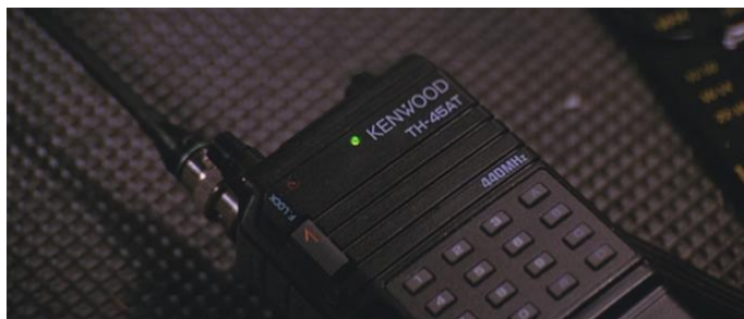
Figure 7. The Kenwood TH-45AT transceiver.
