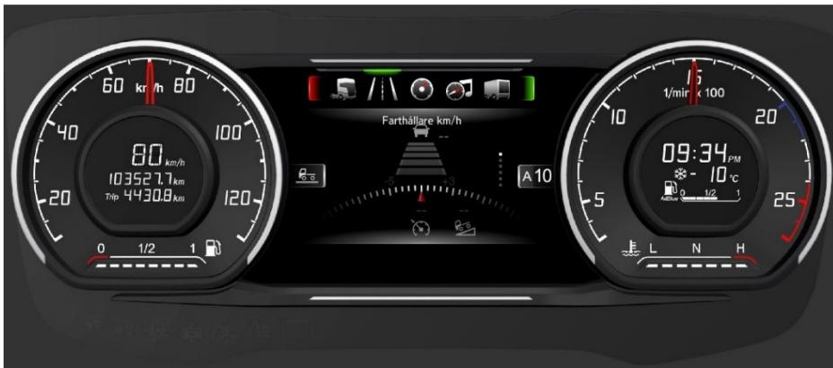
Figure 4.4 Digital interactive prototype of Instrument Cluster from 2013.
