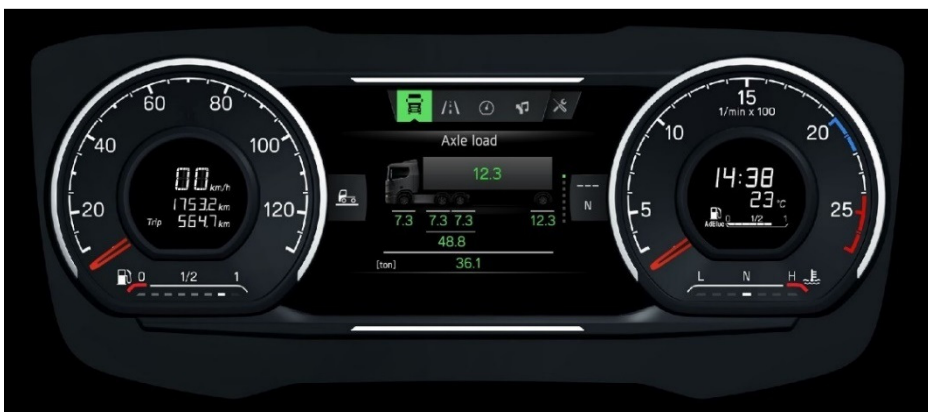
Figure 4.5 Digital interactive prototype of Instrument Cluster from 2015.
