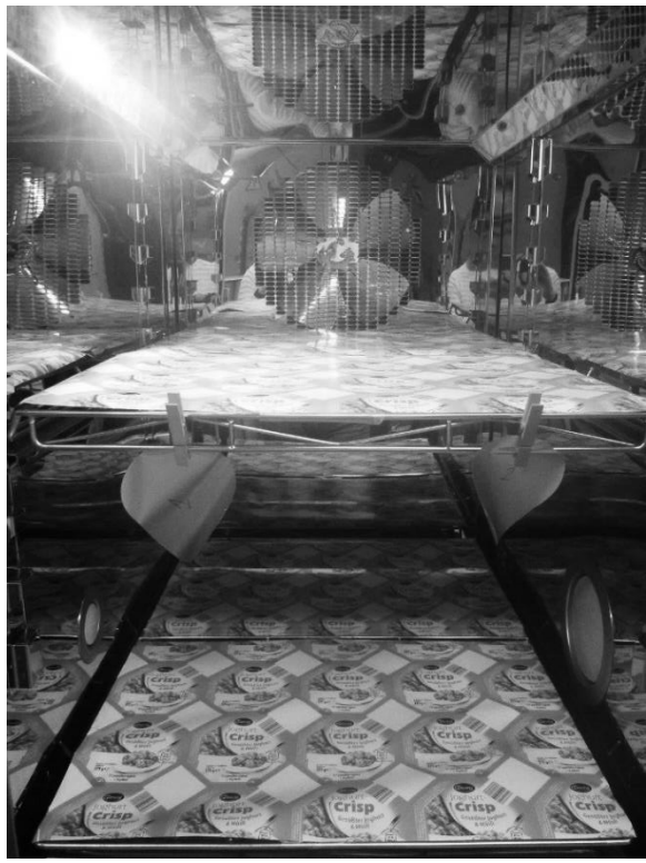
Figure 3.16 Picture of the 4 packaging material sheets and 100-cm 2 circular samples inside the climate chamber at t 0 .
