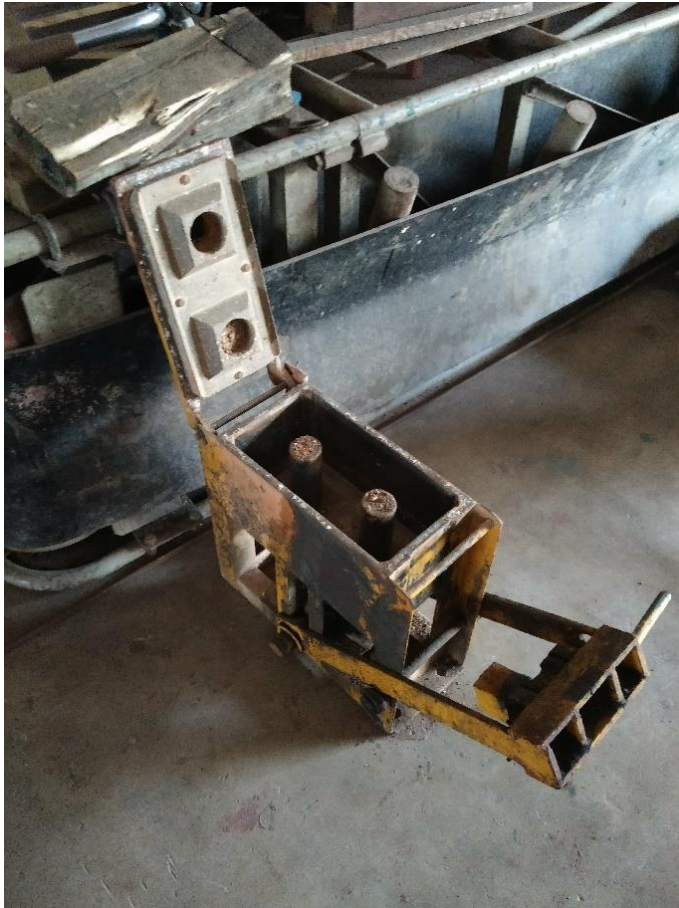
Figure 10 Manually operated machine for single block production
