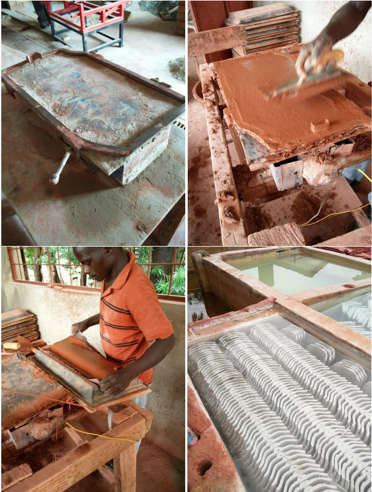
Figure 13 Process of roofing tile production, tile plate form (A), vibrator mix (B), tile moulder (C) and drying and curing (D)
