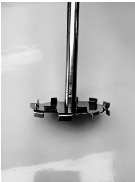
Figure 5.3: High speed disc impeller used for pre-mixing of pigment dispersions.
