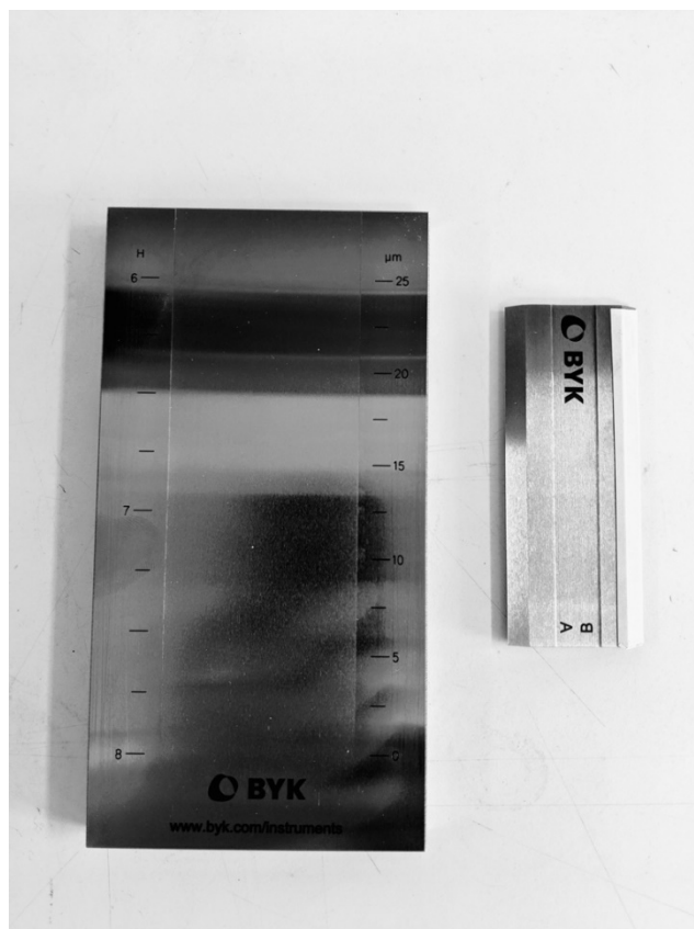
Figure 5.4: Grind gage which can show particles from 0-25 \mu\text{m} .
