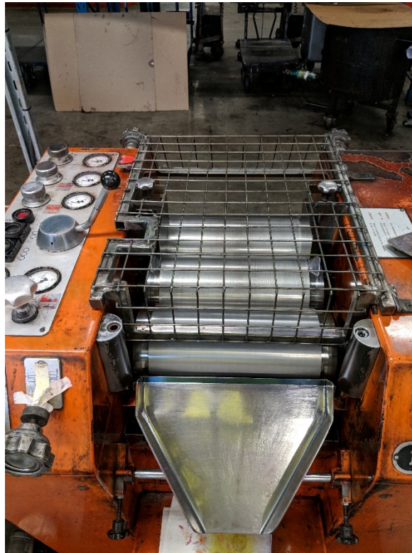
Figure 3.1: A pilot scale three-roll mill used at Flint group.
