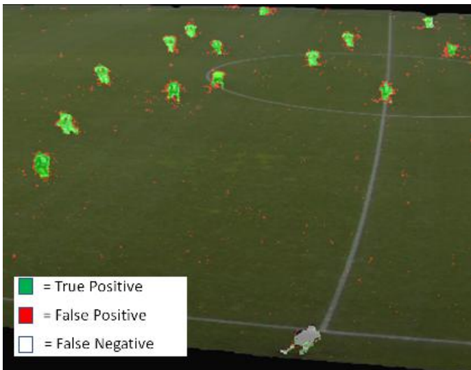
Figure 3.12: Segmented pixels were classified as True Positive, False Positive and False Negative when compared with the ground truth. Note that True negative pixels are shown as transparent.
