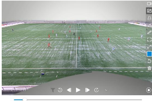
Figure 1.1: A screen-shot from the Spiideo mobile application. The user has the ability to play, pause and use the time-line to navigate between game-play events. The user can also pan, tilt and zoom, or use the drawing tools shown on the right side of the image.
