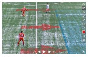
Figure 2: Some conditions causes the current background foreground segmentation to fail. This leads to drawings that are incorrectly presented on top of the foreground or behind the background.
