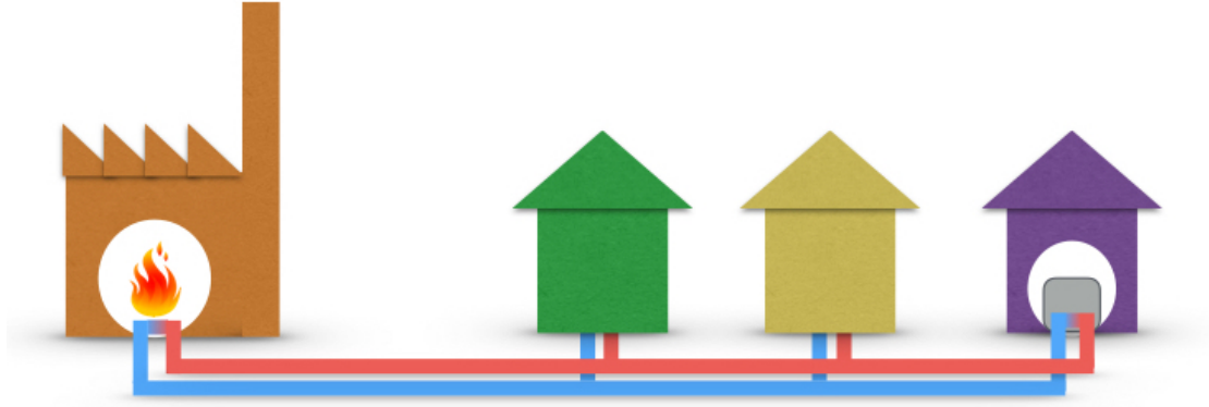
Figure 1: A conceptual image of a simple district heating system. The red and blue lines represent the hot and cold water that is circulated from production site to the customer buildings and back.
