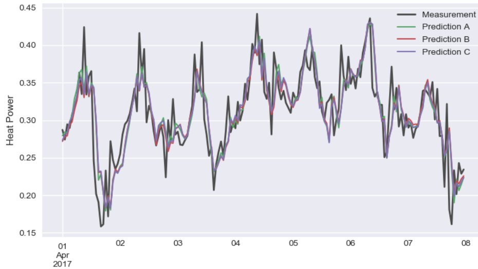
Figure 9: 1-step predictions of the Heat Power (normalized) based on model A, B and C for a typical week in the test set, compared to the actual data.
