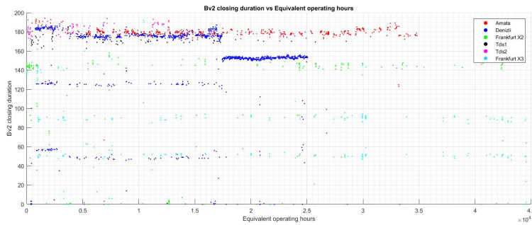
Figure 35: Data point 3, Duration for Bleed valve 2 (BV2) to close during start, plotted equivalent operating hours
