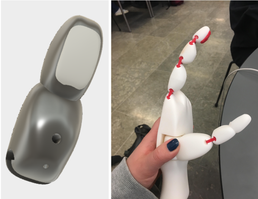
Figure 23: The first prototype of the thumb with only one flexible joint. The CAD model to the left and the printed model to the right.
