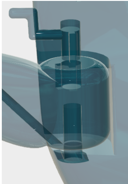
Figure 22: The pivot joint connecting the thumb to the palm, with the locking mechanism in unlocked position.
