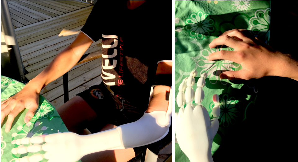
Figure 40: The final prosthesis tested by the patient showing the good size and resemblance to the right arm.
