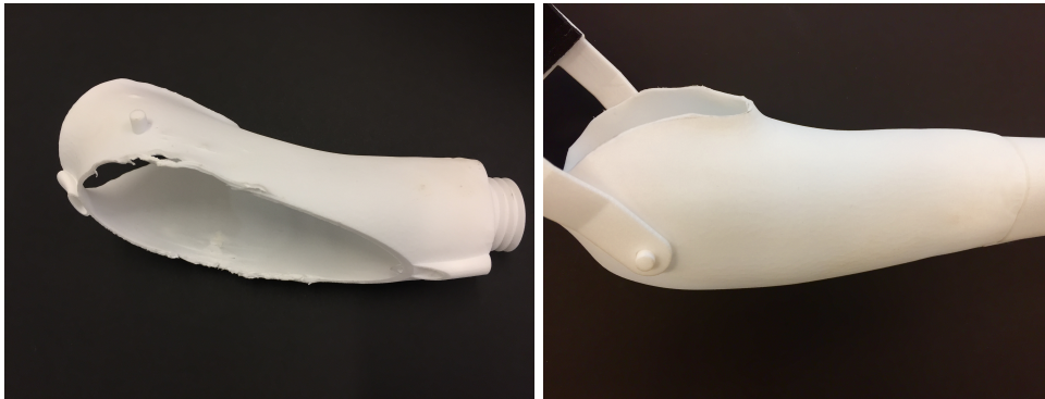
Figure 28: Two sets of the printed prototypes of the socket. Left: The first print failed due to problems in the printer. Right: The final prototype.
