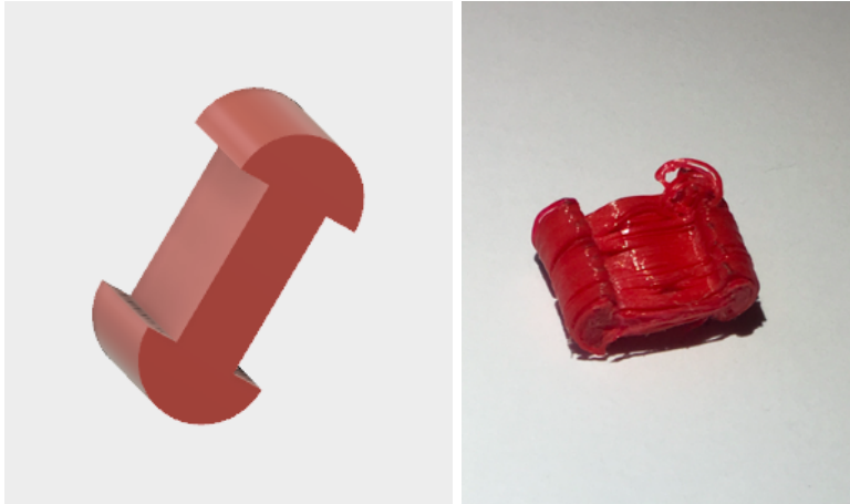
Figure 29: The design of the first version of the elastic joint from Fusion 360 and the second failed attempt of the FDM printed model.
