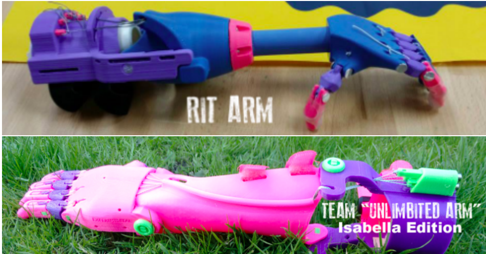
Figure 15: 3D printed transradial prostheses using flexion of the elbow to control the contraction of the hand. Many of the open source prostheses are intended for children and therefore have a playful design, such as the RIT Arm and Team Unlimbited Arm, both from E-nable [33].
