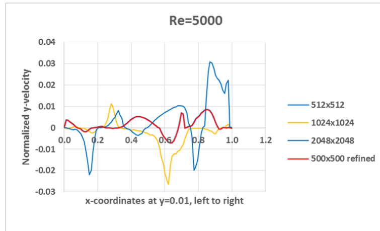
Figure 9: Velocity profile Re=5000 at line 2.
