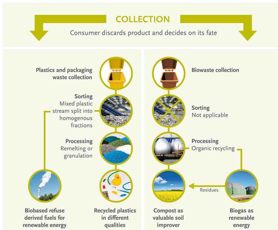
Figure 19. Two separate collection streams for bioplastics, one for mechanical recycling (left) and one for organic recycling (right) (European Bioplastics e.V. 2016b)
