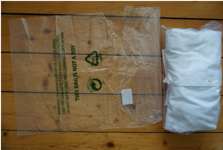
Figure 14. Folding guidelines of garments can reduce the required size of the individual polybag and result in less used plastic material. A shirt is here folded to a smaller size than it “normally” is when packed in an individual polybag. Done with inspiration from Cohen (2014) (photo: Marcus Malmsjö).
