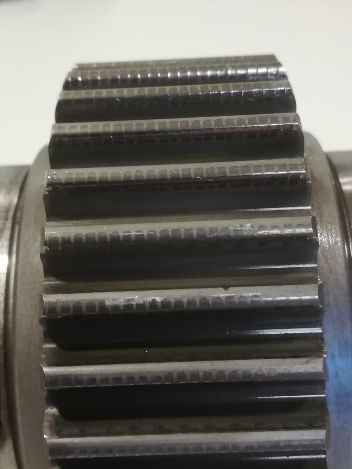
Figur 42. Sprocket with contact fatigue
