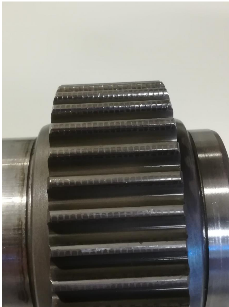
Figure 41. Piano teeth, arising from fatigue
