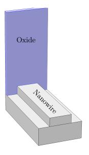
**Figure 4.4:** Side view of nanowire model geometry
