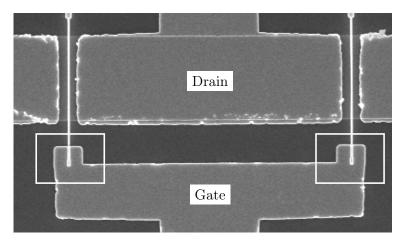
**Figure 4.3:** Finished gate contact layout with extended gate pad sections
