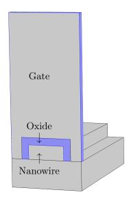
**Figure 4.5:** Gate view of nanowire model geometry
