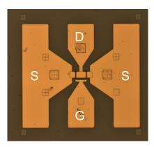
**Figure 3.7:** Pad layout of device type *A*
