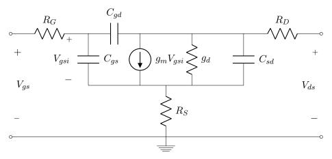
**Figure 5.4:** A hybrid- $\pi$  model of a MOSFET
