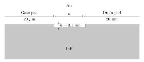
Figure 4.1: Model geometry for the pad capacitance simulation
