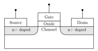
Figure 2.1: Schematic of a planar n-type MOSFET structure.
