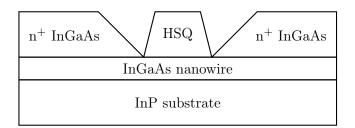
Figure 3.9: Contact growth schematic with HSQ dummy gate
