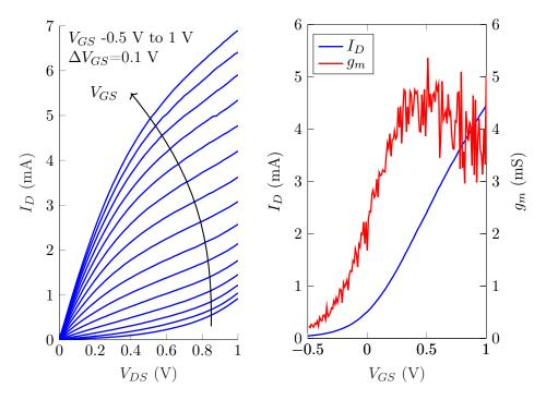
**Figure 6.8:** Output characteristics.
