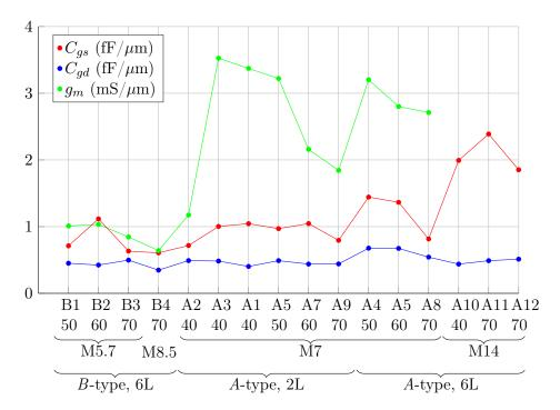
**Figure 6.12:** Transconductance and capacitances for the devices measured on sample V. Device name and gate and mesa dimensions are showed underneath the plot.
