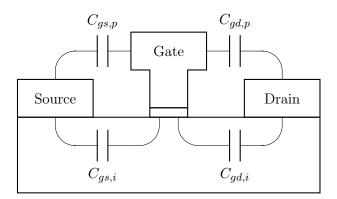
**Figure 5.3:** Schematic describing the intrinsic and parasitic capacitances in MOSFET structure.
