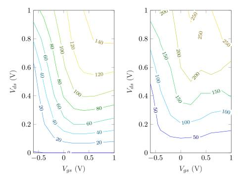
Figure 6.17: Contour plot of  $f_T$
