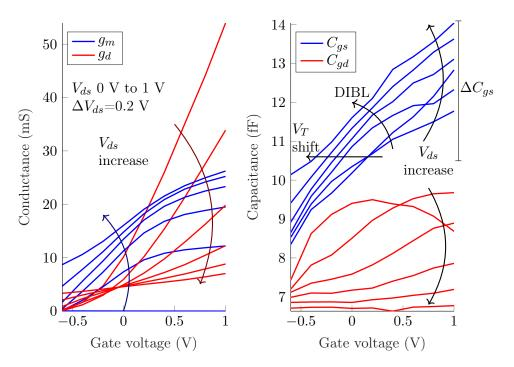
**Figure 6.10:** Extracted transconductance and output conductance for each bias
