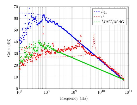
Figure 6.15: Current and power gain.
