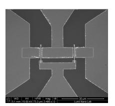
Figure 6.1: A overview of a finished A device with mesa 7  $\mu$ m
