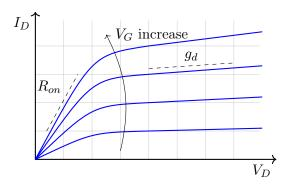
Figure 5.2: Output characteristics.
