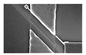
Figure 6.6: SEM image of a misaligned B-device
