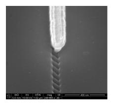
Figure 3.12: A 52° tilted SEM image of a T-gate
