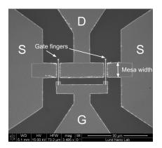
**Figure 3.2:** SEM overview image of a finished *A*-device with source (S), drain (D), gate (G) and mesa width marked
