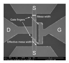
**Figure 3.6:** SEM overview image of a finished *B*-device with source (S), drain (D), gate (G), mesa width and effective mesa width marked. This layout also applies to the *C*-devices.
