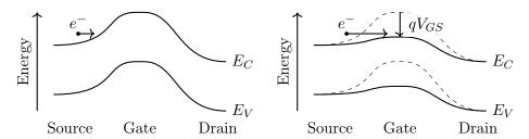
**Figure 2.2:** MOSFET band structure in the off-state
