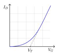
Figure 5.1: Transfer characteristics.
