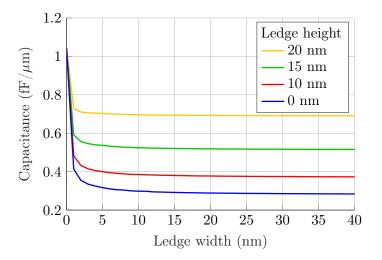
**Figure 4.9:** Gate to source capacitance for different ledge heights and widths
