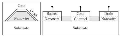
Figure 2.4: Nanowire MOSFET structure
