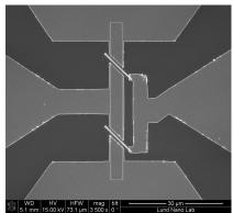
**Figure 6.2:** A overview of a finished B device with mesa 3.5  $\mu$ m
