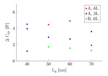
Figure 6.13:  $\Delta C_{qs}$  against gate length
