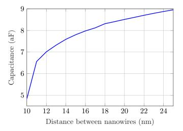
Figure 4.6: Parasitic capacitance per nanowire
