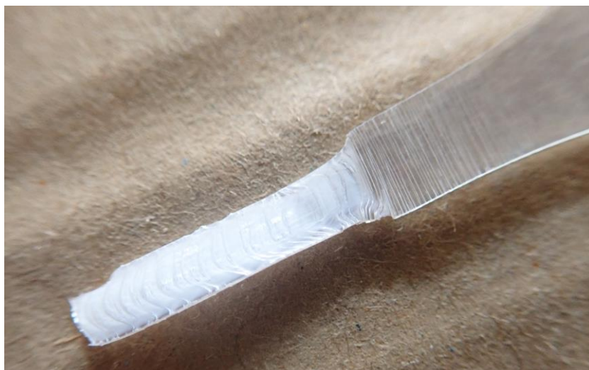
Figure 71. Closer look at the flow pattern in CD, grade 3 after stored 6 weeks. A clear pattern can be seen in the elongated part.
