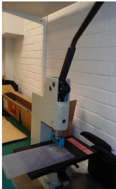
Figure 20. Punching device, where all dogbones been punched by hand.
