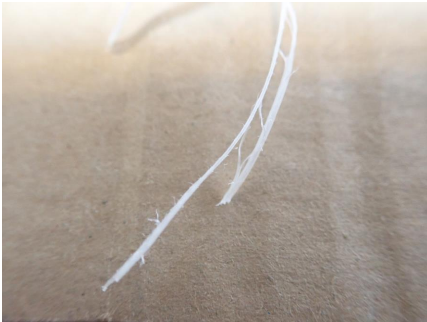
Figure 73. Closer look at the elongated area close to the point of break, in DD, grade 3 stored 6 weeks. The area is not smooth and it looks like fibre has been formed.
