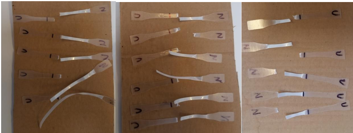
Figure 38. Tensile tested dogbones, punched:(left) 0 mm, (middle) 5 mm, (right) 10 mm from the edge of the plate. The middle of the plate is marked by a line.
