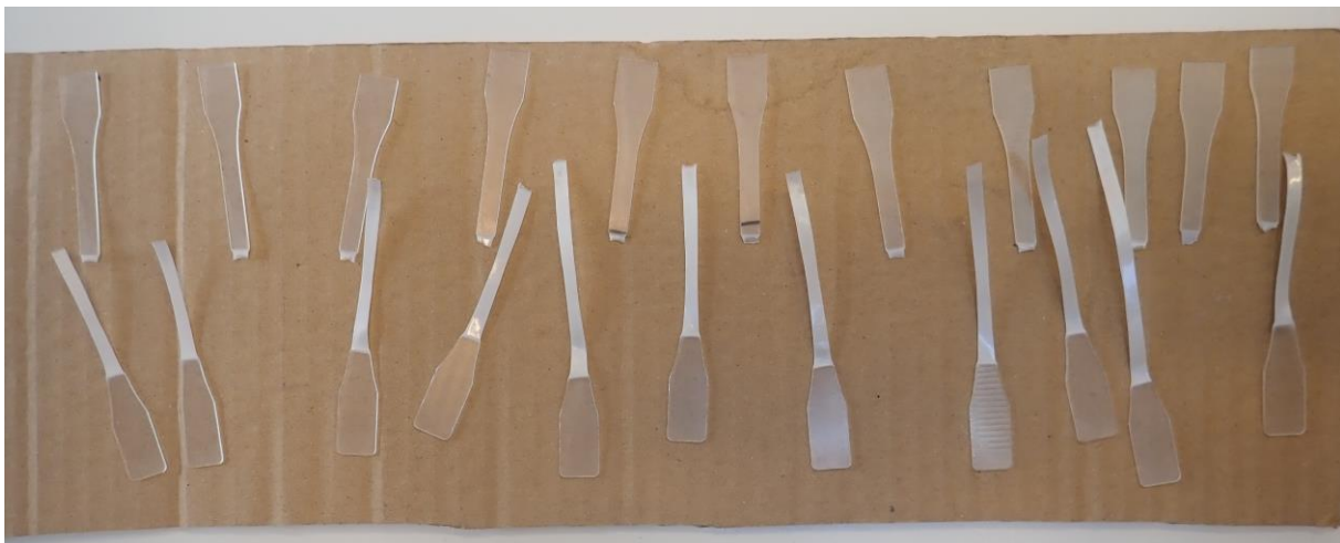
Figure 68. Dogbones after tensile test when elongation and broken in MD by grade 3, when stored in 6 weeks. This elongation is shorter than the one in DD, but longer than the general, stable, break in CD.
