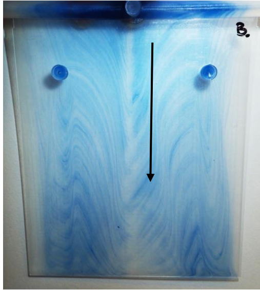
Figure 19. The resulting flowlines when injection moulding the plates, seen by the addition of a pigmented pellet. Orientation of polymer is marked with an arrow. Injection point is outside of picture, on top of the plate (one injection point).
