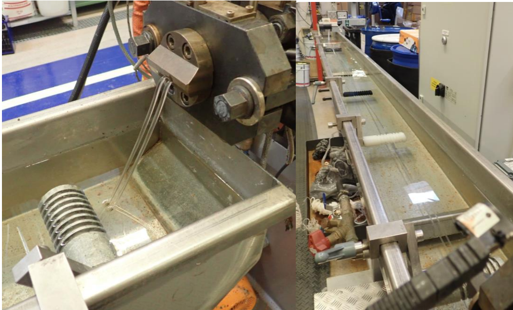
Figure 16. Picture of the molten compounded polymer coming out from the extruder, to be cooled in the water bath of cold tap water.
