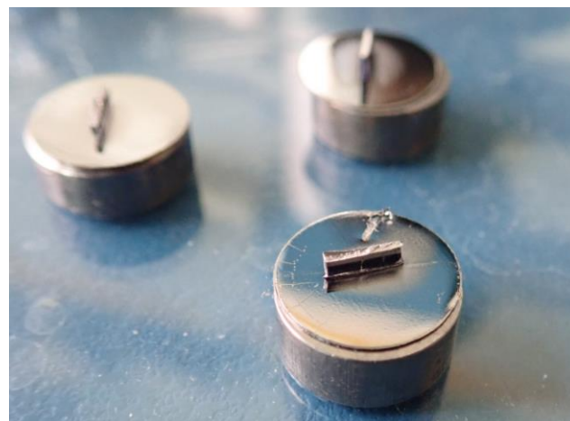
Figure 27. Specimen holder with polymer on top with the surface of interest facing upwards. The specimen and holder have been sputtered with a 15 nm thick layer of palladium/gold (80/20).
