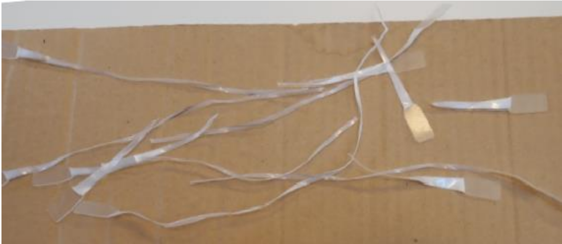
Figure 72. Dogbones after tensile test in DD by grade 3, when stored in 6 weeks. The elongation in DD is longer than the elongation in MD and CD by stable homo-PP.
