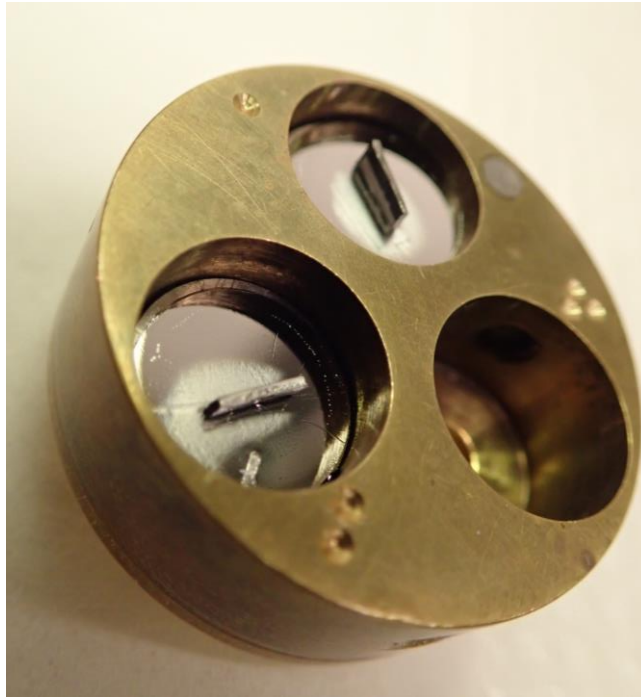
Figure 28. Specimen with specimen holder, where the surface of interest (due to the notch) is placed in towards the centre of the holder.
