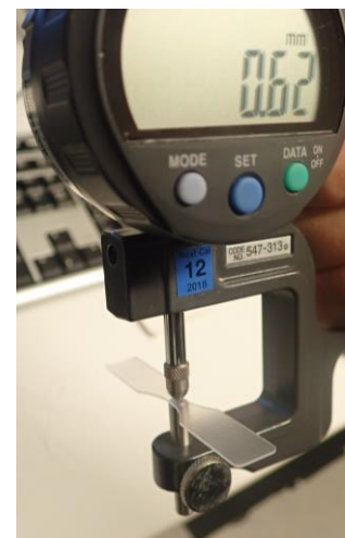
Figure 23. Measuring equipment to determine the thickness of the dogbones used in tensile impact testing.
