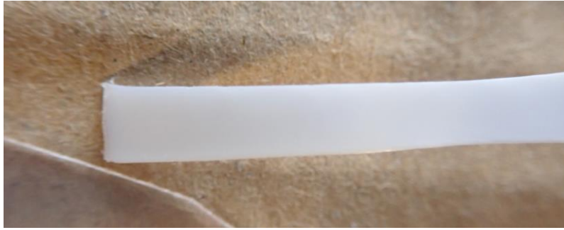
Figure 69. Closer look at the elongated, necked, area in MD, by grade 4 stored 6 weeks. There are no flow lines of polymer to be observed, the polymer is homogeneous white.
