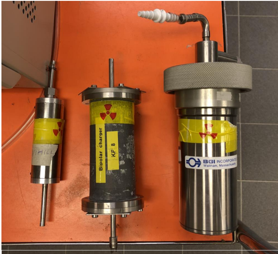
Figure 14. A presentation of the dimensions of Ni-charger, Kr-charger and \alpha -charger. Picture was taken by the author of this thesis (2018).
