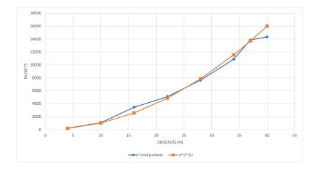
**Figure 6.1:** Total packets between all orderers based on amount of orderers, when the consensus algorithm agrees on the ordering of a new block.  $n^2 \cdot c$ , c = 10 for reference.
