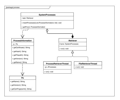
Figure 5.5: UML of the process Java package.
