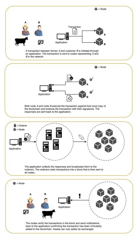
Figure 2.11: The transaction flow in Fabric v1.0
