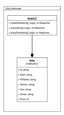
Figure 5.3: UML of the VoteCC.go chaincode and the JSON structure defined by it.
