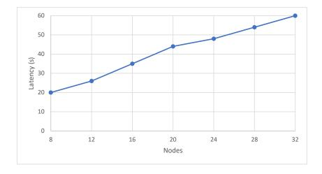
Figure 7.3: Latency in Fabric v0.6 with 8 clients and an increasing number of nodes.
