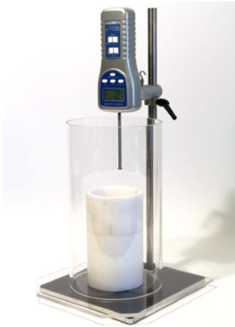
Figure 3. Force gauge meter with accessories for measuring headspace volume
