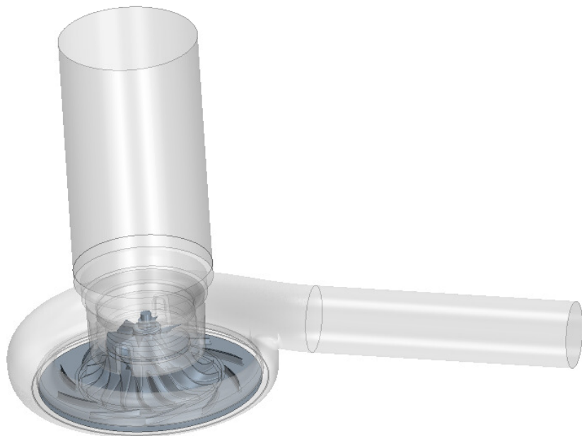
Figure 1. The complete model of the in-house-compressor in Star-CCM+.
