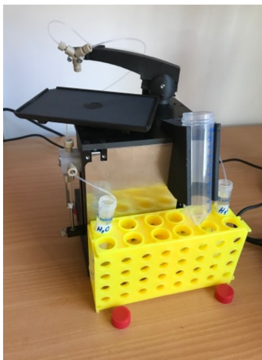
Figure 1: The dispenser machine, Gradis that was used in the experiments. The channels A and B start with small tubes that are placed in the selected samples. The machine pumps the liquid from the sample containers (in front of the machine) into the syringes (on both sides of the machine) while loading them and then selected volumes of the samples are pumped through the dispenser head (on top of the machine) and dispensed into the wells of a 96-well plate (on the black rotating platform). The large Falcon tube (in front of the machine) is the waste collector, where flush volumes and switch volumes are dispensed.
