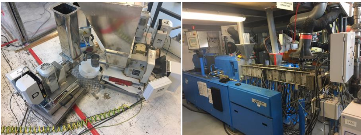
Figure 19. Figure showing the extrusion setup at Fraunhofer ICT. Hopper (left) and extruder (right) [40].
